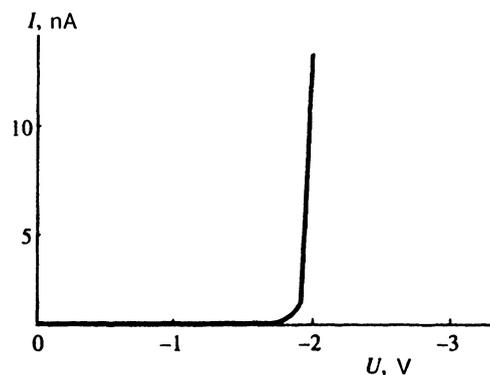
FIG. 2. Current-voltage characteristic of sample No. 1 with layer thickness  $d=4.5$   $\mu\text{m}$ ;  $T=10.0$  K,  $S=50 \times 50 \text{ } \mu\text{m}^2$ .
