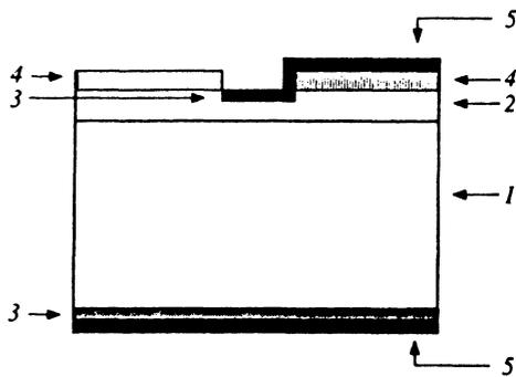
FIG. 1. Cross section of the experimental structures. 1—Strongly doped silicon substrate, 2—epitaxial layer, 3—contact regions, 4—dielectric layer, 5—metal.
