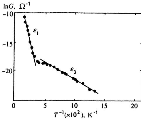
FIG. 3. Temperature dependence of the conductivity for sample No. 2 with epitaxial layer thickness  $d=4.5 \mu\text{m}$ ,  $S=50 \times 50 \mu\text{m}^2$ .
