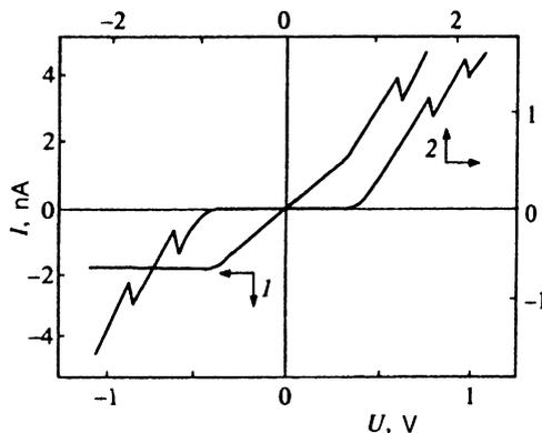
FIG. 4. Current-voltage characteristics of samples with a layer of thickness  $d=4.5 \mu\text{m}$ ,  $S=50 \times 50 \mu\text{m}^2$ . 1—Sample No. 2,  $T=15.0 \text{ K}$ , 2—sample No. 3,  $T=11.6 \text{ K}$ .
