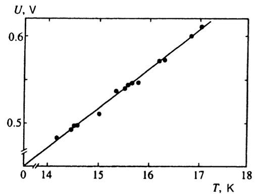
FIG. 5. Temperature dependence of the position of a negative differential resistance peak for sample No. 2.  $d=4.5 \mu\text{m}$ ,  $S=50 \times 50 \mu\text{m}^2$ .
