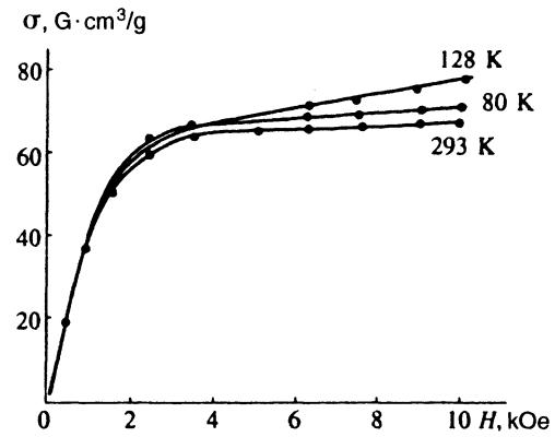
FIG. 6. Isothermal curves of magnetite magnetization taken at temperatures of 293 K, 80 K, and around  $T_f$  at 128 K in magnetic fields of up to 10 kOe.
