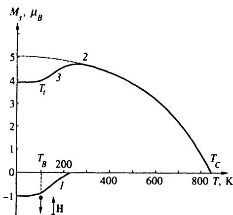
FIG. 5. Curves of magnetite magnetization versus temperature in the low-temperature range: (1) magnetization of the weak sublattice; (2) sum magnetization of the combined  $BA$ -sublattice; (3) total magnetization.
