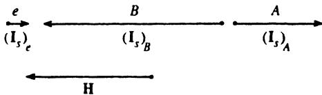
FIG. 4. Magnetic structure of magnetite at temperatures below  $T_f$ ;  $(\mathbf{I}_s)_e$ ,  $(\mathbf{I}_s)_B$ , and  $(\mathbf{I}_s)_A$  are the spontaneous magnetizations of the weak, octahedral, and tetrahedral sublattices, respectively.
