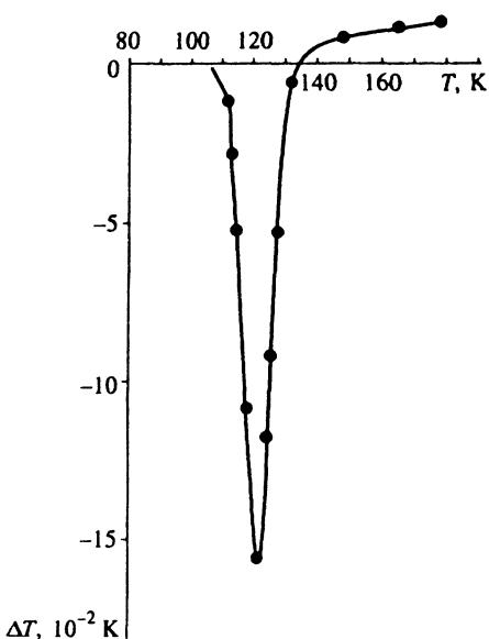
FIG. 1. Maximum of the negative  $\Delta T$ -effect near  $T_t$  at  $H = 10 \text{ kOe}$  plotted from the data of Ref. 8.
