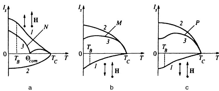
FIG. 3. Spontaneous magnetization of (1) weak and (2) strong sublattices as functions of temperature, and (3) Néel's (a)  $N$ -, (b)  $M$ -, and (c)  $P$ -curves of  $I_s(T)$ . The arrows near the curves 1 show the alignment of the weak sublattice magnetic moment with respect to external magnetic field.
