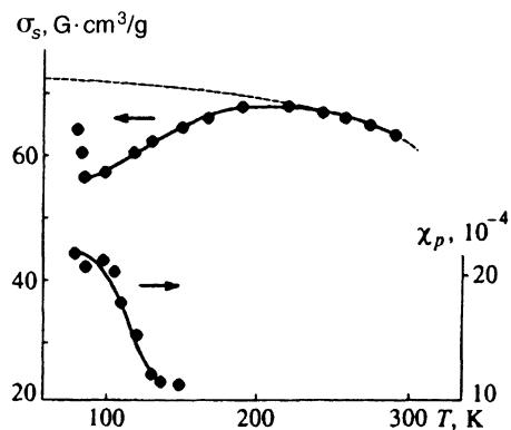
FIG. 2. Anomalies of the spontaneous magnetization  $\sigma_s$  and susceptibility of the paraprocess  $\chi_p$  near  $T_i$ , plotted from the data of Ref. 9.
