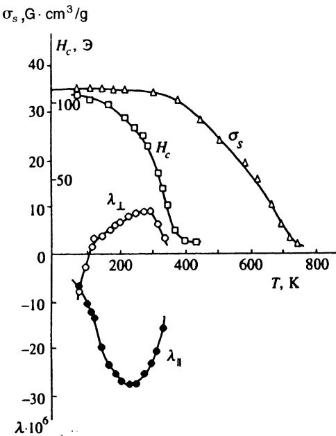
FIG. 1. Spontaneous magnetization  $\sigma_s$ , coercive force  $H_c$ , perpendicular  $\lambda_\perp$  and parallel  $\lambda_\parallel$  magnetostricitions as functions of temperature measured under a magnetic field  $H = 10$  kOe.
