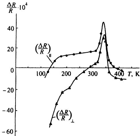
FIG. 4. Transverse  $(\Delta R/R)_{||}$  and longitudinal  $(\Delta R/R)_{\perp}$  relative magnetoresistances as functions of temperature measured at  $H=10$  kOe.
