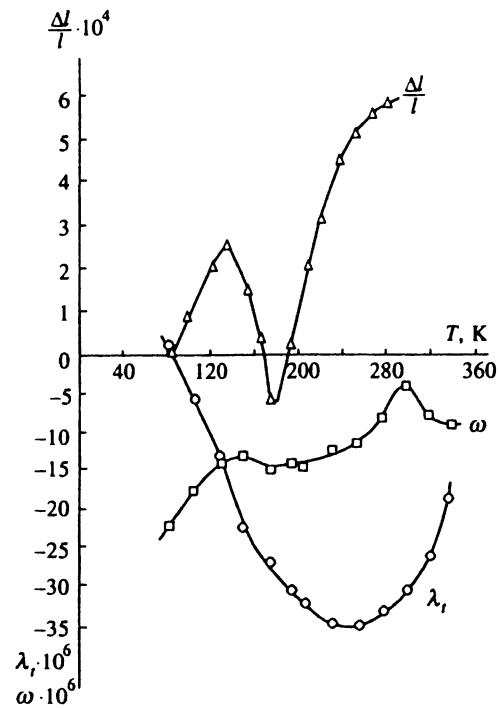
FIG. 2. Anisotropic  $\lambda_t$  and volume  $\omega$  magnetostricitions versus temperature measured at  $H = 10$  kOe and relative thermal expansion  $\Delta l/l$ .
