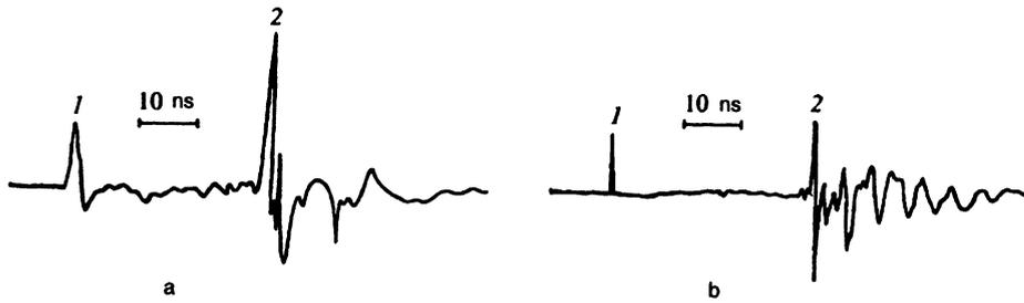
FIG. 1. Typical oscillograms of the laser pulse (1) and the current pulse of the high-energy electrons from the plasma (2): a) heating of the plasma by a nanosecond laser pulse; b) heating of the plasma by a picosecond laser pulse. The amplitudes of the positive pulses 2 correspond to 320 keV (a) and 30 keV (b).
