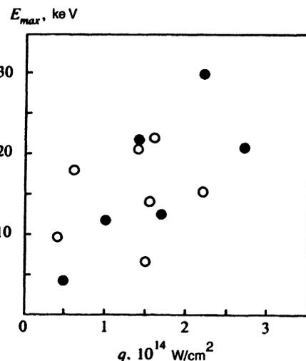
FIG. 3. Dependence of the maximum energy of the high-energy electrons on the flux density of the laser radiation on the target for an aluminum plasma heated by a picosecond laser pulse; the open circles and black circles are for  $p_1 = 10^{-2}$  torr and  $p_2 = 10^{-5}$  torr, respectively.
