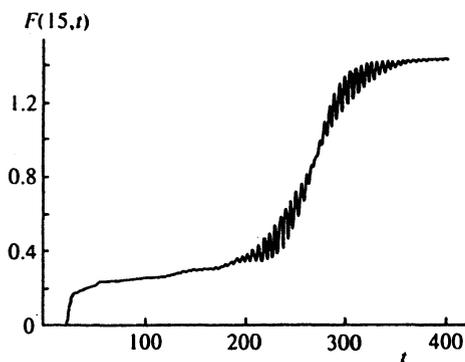
FIG. 8. Energy flux through the plane  $x_f=15$  plane as a function of time for a long-lived resonant structure. The field of the escaping kink is strongly perturbed, as is seen from the flux oscillations. The initial kink velocity was  $V=0.7646$ .
