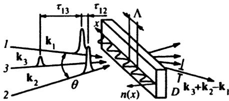
FIG. 1. Basic arrangement of the three-beam experiment on laser-induced gratings.
