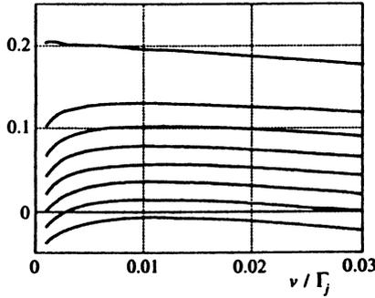
FIG. 3. The  $\nu/\Gamma_j$ -dependence of the relative narrowing of the absorption spectrum  $\mathcal{P}^{(1)(1)}(\Omega, \Omega_\mu)$  as  $\Omega$  varies from 0 to  $kv_T$  (for  $\kappa_\mu = -1$ ), obtained as a result of numerical calculations by Eq. (21). The different curves correspond to different values of  $\Gamma$ , from  $\Gamma=0$  (the upper curve) to  $\Gamma=7 \times 10^{-2} kv_T$ , with a growth rate of  $10^{-2} kv_T$ .
