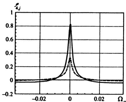
FIG. 4. The shape of the peak corresponding to two-photon processes for  $\Gamma = 10^{-2} kv_T$ ,  $\Omega = 0$ , and  $\Gamma_j = 10^{-3} kv_T$  with  $\nu = 10^{-3} kv_T$  (the solid curve) and  $\nu = 10^{-4} kv_T$  (the dashed curve), in arbitrary units.
