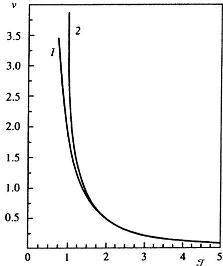
FIG. 6. Dependence of the power of a pulse on its duration for a medium with inhomogeneously broadened absorption line. Curve 1 corresponds to the effect of “pure” self-induced transparency. Curve 2 takes into account the presence of nonresonant nonlinearity:  $\nu \neq 0$ . Instead of the power, the ordinate gives the dimensionless parameter  $\nu$ , which is proportional to the power.
