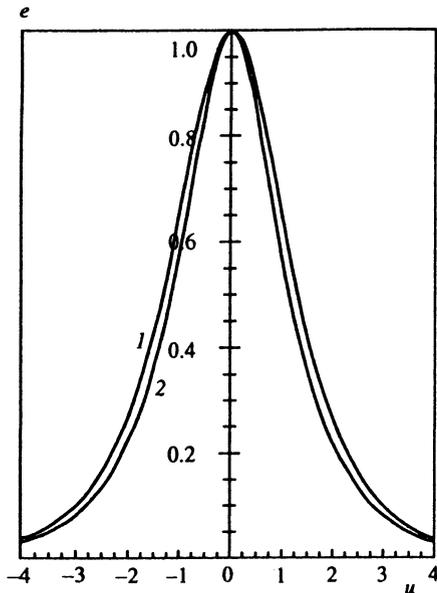
FIG. 1. Shape of pulse envelope  $e(u)$ . Curve 1 represents the “pure” effect of self-induced transparency; the same shape is obtained in perturbation theory (for small values of  $\nu$ ). Curve 2 gives the exact theory based on the combined effect of self-induced transparency and phase self-modulation,  $\nu=2\sqrt{2}$ .
