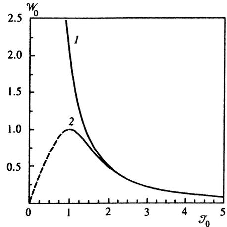
FIG. 2. Graph of dependence of the power of a pulse on its duration. Curve 1 corresponds to the effect of “pure” self-induced transparency:  $\nu=0$ . Curve 2 takes into account the existence of nonresonant nonlinearity:  $\nu \neq 0$ . The dashed curve is the branch corresponding to the unstable solution. The power and duration are normalized in accordance with (26).
