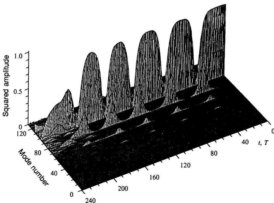
FIG. 5. Evolution of waves in an FPU lattice. A carrier wave with  $k = 3\pi/4$  (mode number 96) and  $\gamma = 0.03$  and a weak perturbative wave with  $Q = \pi/8$  (mode number 80) were excited at the onset.
