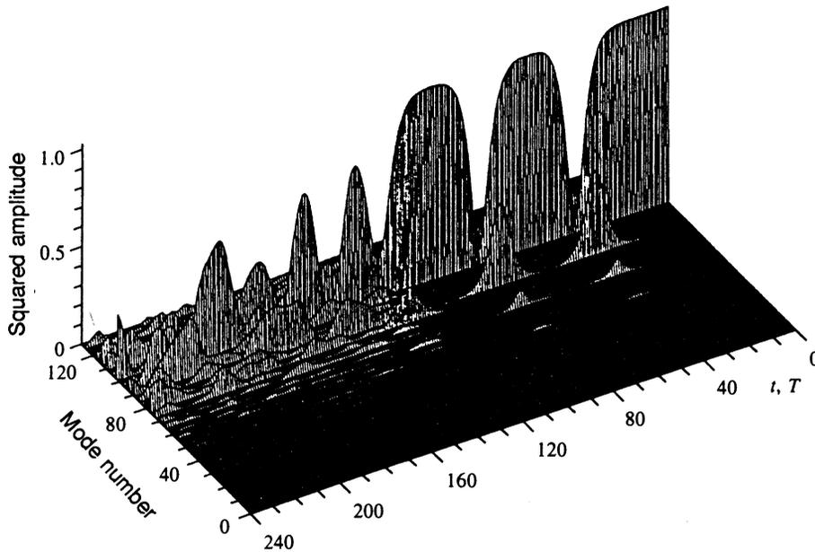
FIG. 6. Evolution of waves in an FPU lattice. A carrier wave with  $k = (3/4 + 1/128)\pi$  (mode number 97) and  $\gamma = 0.03$  and a weak perturbative wave with  $Q = \pi/8$  (mode number 81) were excited at the onset.
