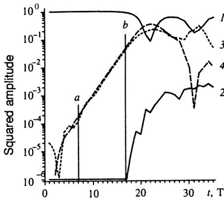
FIG. 1. Behavior of the squares of the amplitudes of a carrier wave with  $k=3\pi/4$  (1), a third harmonic (2), and satellites of the carrier wave having the wave vectors  $k\pm Q$  with  $Q=14\pi/128$  (3 and 4, respectively). The segment  $ab$  corresponds to an exponential increase in the amplitude of the satellites.
