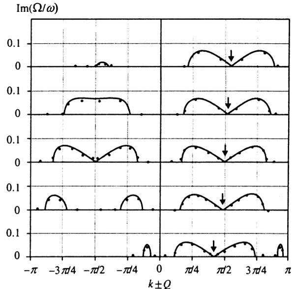
FIG. 3. The growth rate  $\Omega''(k,Q)/\omega$  for wave vectors of the carrier wave (their values are indicated by the arrows) in the vicinity of  $\pi/2$ . Curves – calculation based on Eq. (5) for  $\gamma=0.1$ ; points – results of the numerical experiment.
