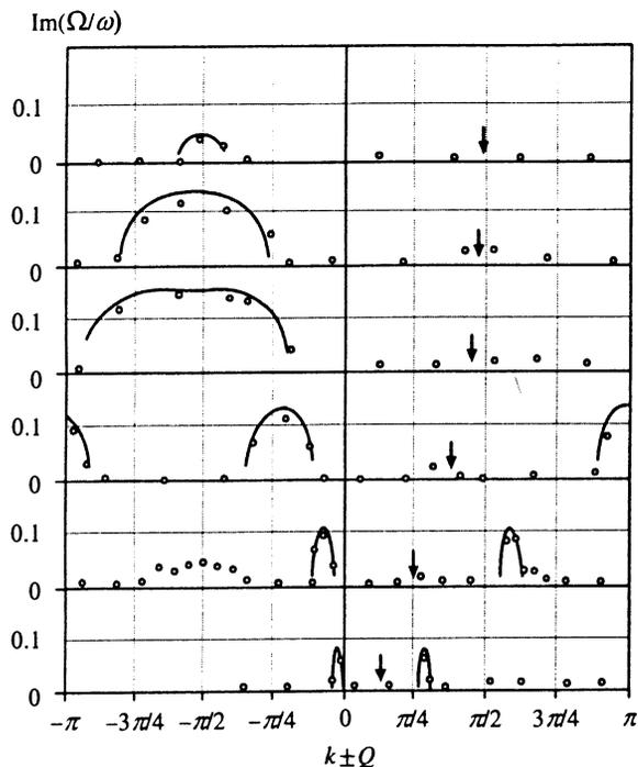
FIG. 4. The growth rate  $\Omega''(k, Q)/\omega$  for wave vectors of the carrier wave (their values are indicated by the arrows) in the vicinity of  $\pi/2$ . Curves – calculation based on Eq. (5) for  $\gamma = -0.1$ ; points – results of the numerical experiment.
