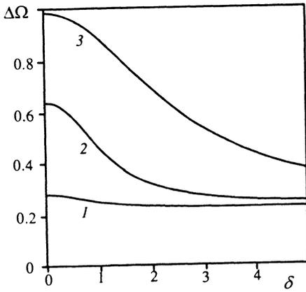
FIG. 5. The halfwidth  $\Delta\Omega$  of the cyclotron resonance peak as a function of the splitting energy  $\delta$  at  $\mu=0.8$  and  $\Omega_T=0.3$  (curve 1),  $\Omega_T=1$  (curve 2), and  $\Omega_T=3$  (curve 3).
