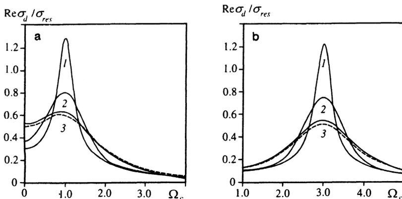
FIG. 4. The shape of the cyclotron absorption peak for the resonant ( $\delta=0$ ) case at  $\mu=0.8$  and  $\Omega_T=0.3$  (curves 1),  $\Omega_T=1$  (curves 2), and  $\Omega_T=3$  (curves 3): (a)  $\Omega=1$ , and (b)  $\Omega=3$ . The dashed curve corresponds to the classical (Drude) peak specified by the "mean" relaxation time  $\tau$ .
