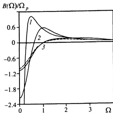
FIG. 7. The proportionality factor  $B(\Omega)$  in the formula for the tangent of the Faraday rotation angle ( $\tan \theta_F = B(\Omega)\Omega_c$ ,  $\Omega_c \rightarrow 0$ ) as a function of the radiation frequency  $\Omega$  at  $\delta=0$ ,  $\mu=0.8$ ,  $\Omega_T=0.3$  (curve 1),  $\Omega_T=1$  (curve 2), and  $\Omega_T=3$  (curve 3). The dashed curve describes the  $B(\Omega)$  dependence calculated by the Drude formula.
