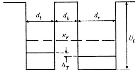
FIG. 1. The band diagram and the position of levels for a model of a double quantum-well structure.
