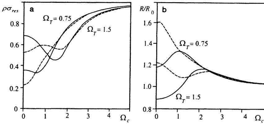
FIG. 3. The magnetic field graphs of the classical magnetoresistance (a) and the Hall constant (b) for the resonant ( $\delta=0$ , solid curves) and nonresonant ( $\delta=1$ , dashed curves) cases at two different values of the tunneling matrix element.
