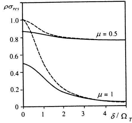
FIG. 2. The shape of the resistivity resonance peak defined by Eq. (36) at  $\mu=0.5$  and  $\mu=1$  for  $\Omega_T=1$  (solid curves) and for  $\Omega_T \gg 1$  (dashed curves).
