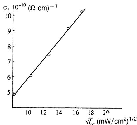
FIG. 2. The electrical conductivity as function of the radiation intensity. The R6G density is  $C=0.63 \text{ mole/l}$ .
