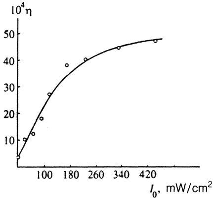
FIG. 4. Diffraction efficiency as function of the total wave intensity.  $U_0 = 1.75$  V;  $\beta = 1.9 \times 10^{-2}$  rad.
