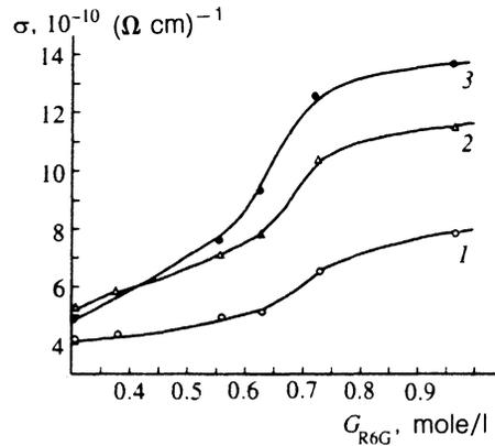
FIG. 1. The electrical conductivity of the mixture as function of the R6G density: 1— $I_0=65 \text{ mW/cm}^2$ , 2— $I_0=165 \text{ mW/cm}^2$ , 3— $I_0=225 \text{ mW/cm}^2$ .
