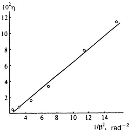
FIG. 5. Diffraction efficiency as function of the intersection angle of the waves in the sample.  $I_0 = 200$  mW/cm<sup>2</sup>;  $U_0 = 1.41$  V.
