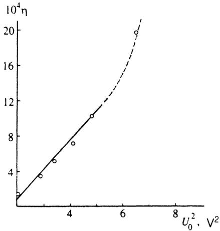
FIG. 6. Diffraction efficiency as function of the voltage applied to the cell;  $I_0 = 180$  mW/cm<sup>2</sup>;  $\beta = 1.9 \times 10^{-2}$  rad.
