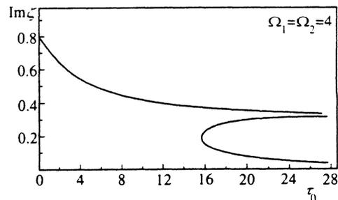
FIG. 6. Evolution of the purely imaginary roots of the scattering coefficient as a function of the time  $\tau_0$  between successive pulses.
