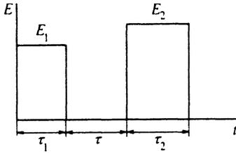
FIG. 1. Shape of the exciting optical pulses applied to the resonant medium.
