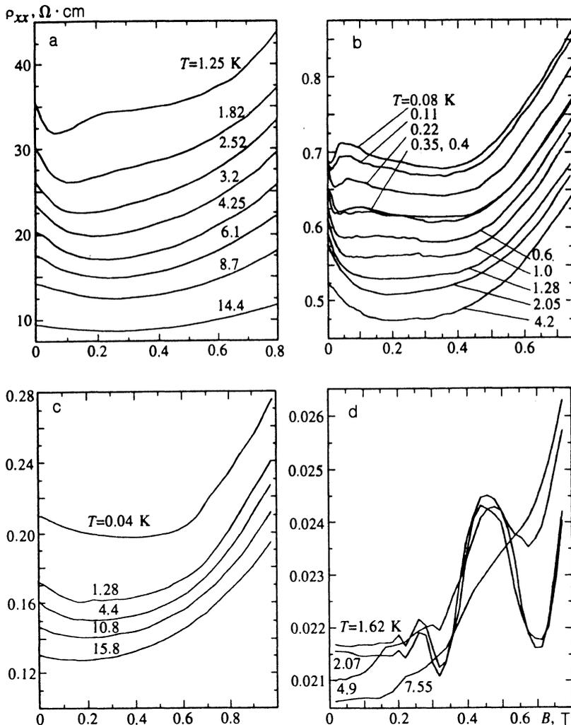
FIG. 1. Transverse resistance as a function of magnetic field for InSb samples No. 14 (a), No. 2 (b), No. 5 (c), and No. 7 (d), at different temperatures.
