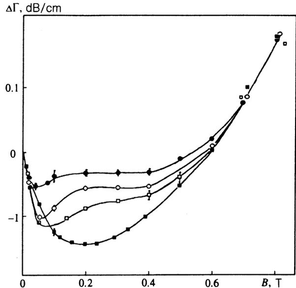
FIG. 8. Magnetic-field dependence of the ultrasonic absorption coefficient for sample No. 2 at different temperatures:  $T=0.46$  K (filled circles), 0.8 K (open circles), 1.2 K (open squares), and 4.2 K (filled squares).
