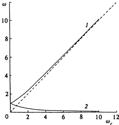
FIG. 1. Magnetoplasmon spectrum of an antidisk in dimensionless units for  $j = |m| - 1$ ;  $m = 1$ ,  $j = 0 (1 - |\omega_-|, 2 - \omega^+)$ .
