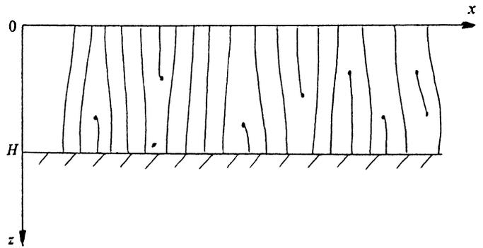
FIG. 2. Typical pattern of constant-phase lines in a cross section of an acoustic waveguide. The lines are spaced at intervals of  $2\pi$ .
