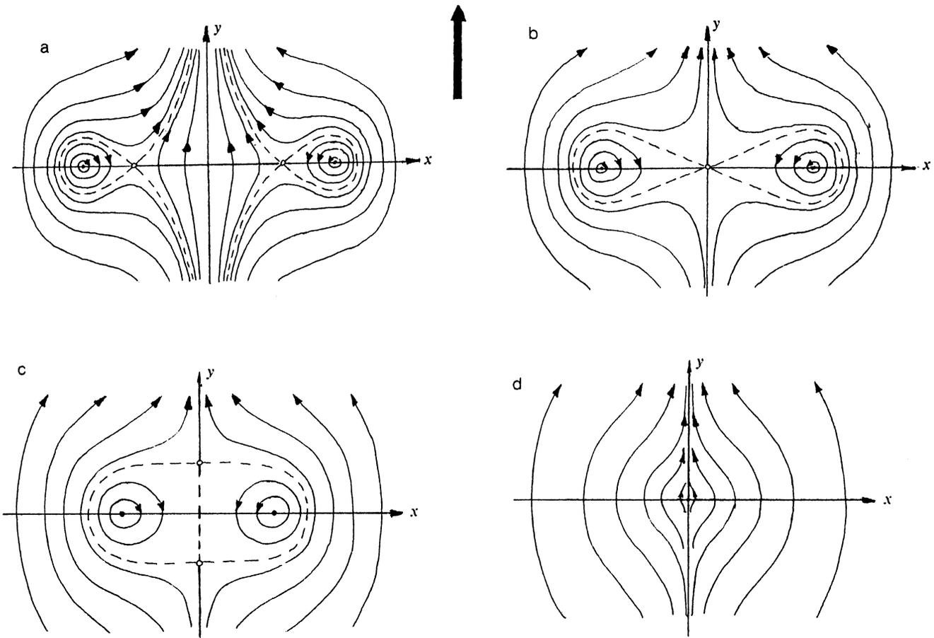
FIG. 1. Energy flux lines near zeros (dots) and saddle points (circles) in the symmetric case. The dashed lines are separatrices. The general energy propagation direction is along the  $y$  axis. a— $\varepsilon=1.5$ ; b—1; c—0.5; d—0.
