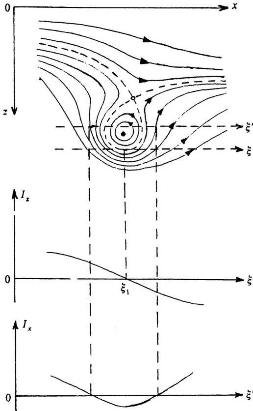
FIG. 3. Behavior of the  $x$  and  $z$  components of the Poynting vector along the horizontals  $\xi$  and  $\xi'$  at a certain distance from a field zero.
