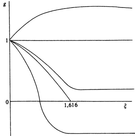
FIG. 1. Schematic form of the scaling functions  $g(\xi)$  [see (13) and (14)] upon application of a constant external magnetic field  $H > 0$ , if the vortices are uniformly distributed at the initial instant over a semi-infinite soft superconductor. Each curve corresponds to a separate value of the magnetic induction in the specimen at the initial instant.
