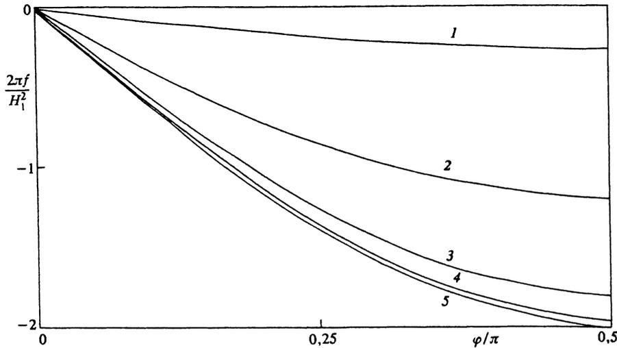
FIG. 6. Dependence of  $f$  [see (28)] on  $\varphi$  for  $H_a(t) = H_1 \sin \omega t + H_2 \sin(2\omega t + \varphi)$ ,  $H_2/H_1 = 0.1, 0.5, 1, 2, 10$ —curves 1, 2, 3, 4, and 5, respectively.
