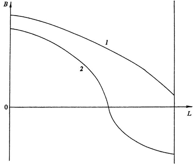
FIG. 3. Schematic diagram of distribution of vortices across a slab in the presence of a constant external magnetic field  $H$  and a current  $J$ . 1— $|H| > 2\pi|J|/c$ , 2— $|H| < 2\pi|J|/c$ .
