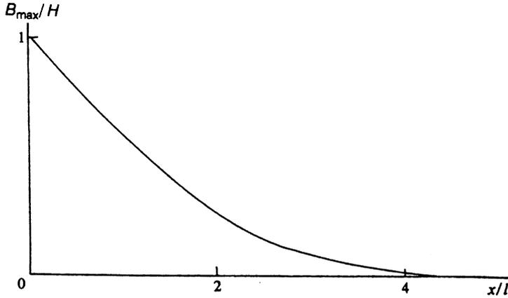
FIG. 8. Coordinate dependence of  $\max_t B(x,t)$  as  $t \rightarrow \infty$ , i.e. amplitude of induction oscillations in a semi-infinite specimen in the steady state.  $H_a(t) = H \sin \omega t$ .
