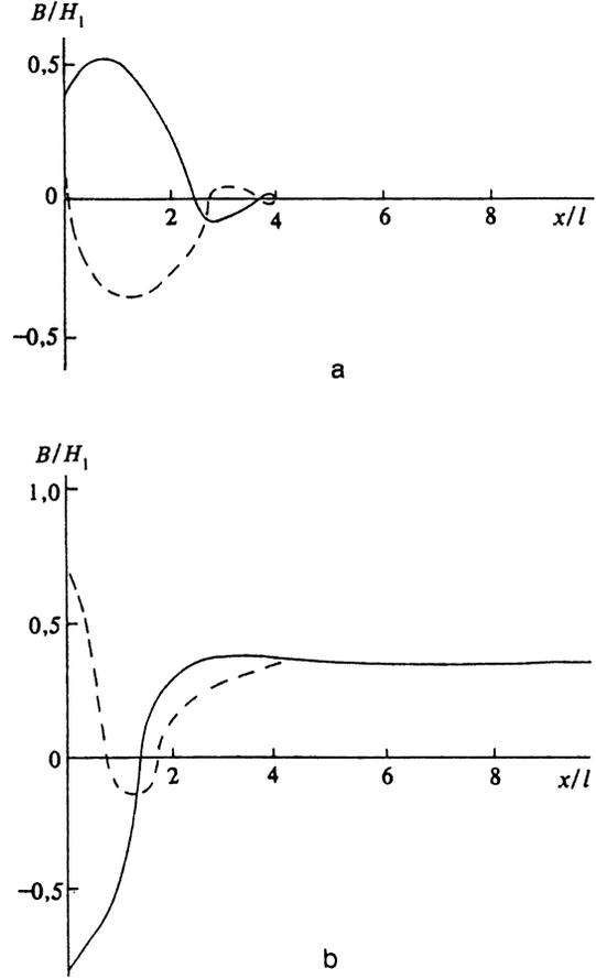
FIG. 4. Instantaneous spatial distributions of the magnetic induction in a semi-infinite specimen ( $x > 0$ ) in the case of a periodic external magnetic field  $H_a(t)$ —results of a numerical solution of Eq. (11). The solid and dashed lines correspond to different instants of time following the end of the initial relaxation. a— $H_a(t) = H_1 \sin \omega t$ , b— $H_a(t) = H_0 + H_1 \sin \omega t$ ,  $H_0/H_1 = 0.1$ . Note that in the last case  $B_\infty$  is considerably stronger than  $H_0$ .
