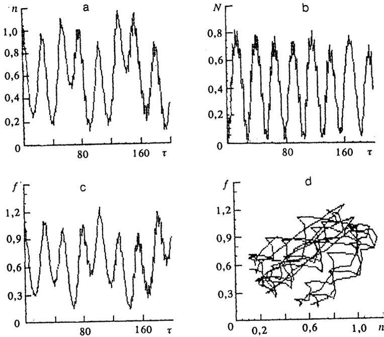
FIG. 5. The time dependence of the number of (a) excitons, (b) biexcitons, and (c) photons, and (d) the projection of the phase trajectory onto the  $(f, n)$  plane at  $n_0=f_0=1$ ,  $N_0=10^{-8}$ ,  $\varphi_{a0}=\varphi_{ph}=1.571$ ,  $\varphi_{b0}=10^{-8}$ , and  $\lambda=0.3$ .
