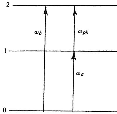
FIG. 1. Energy diagram of one-photon conversion of an exciton into a biexciton: 0 is the ground state of the system, 1 the excitonic level, 2 the biexcitonic level,  $\omega_{ph}$  the excitation frequency,  $\omega_a$  the exciton transition frequency, and  $\omega_b$  the biexciton transition frequency.
