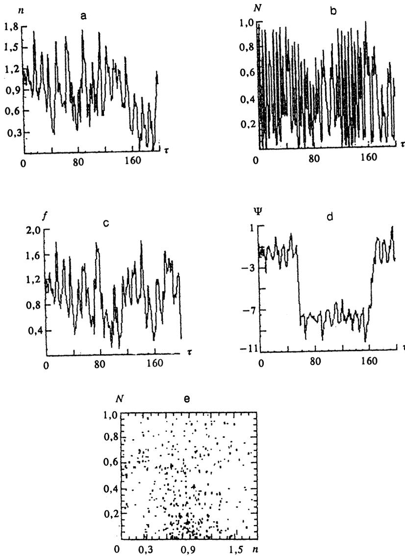
FIG. 6. Expanded stochastic mode of oscillations of (a) coherent excitons, (b) biexcitons, (c) photons, and of (d) the phase, and (e) the phase portrait in the  $(n, N)$  plane at  $n_0=f_0=1$ ,  $N_0=10^{-8}$ ,  $\varphi_{a0}=\varphi_{ph}=1.571$ ,  $\varphi_{b0}=10^{-8}$ , and  $\lambda=2$ .
