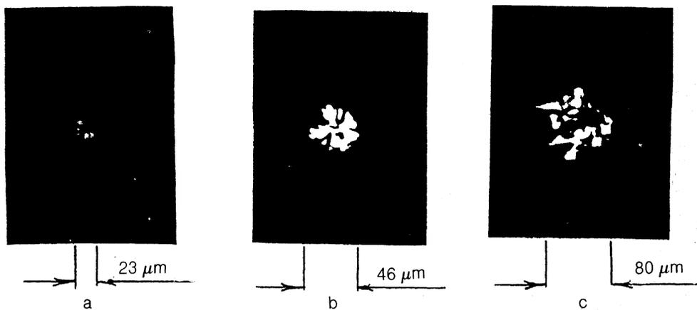
FIG. 4. Photographs (taken through the Polam L-213) of distortions caused by a narrow light beam in the smectic phase of an OCBP liquid crystal (with a thickness  $L_2=40 \mu\text{m}$ ). a— $P\sim 200 \text{ mW}$ ; b— $\sim 270$ ; c— $\sim 380 \text{ mW}$  (crossed polarizers).
