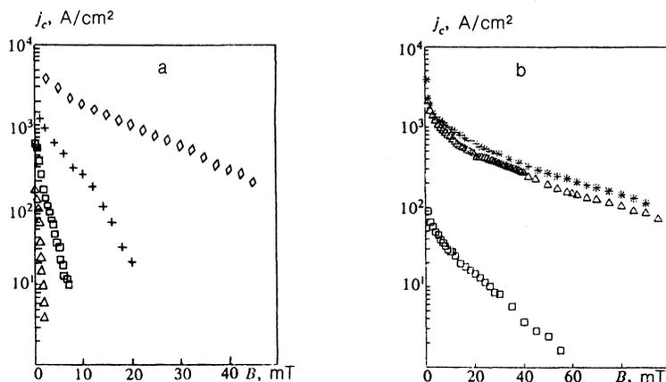
FIG. 7. a) Field dependences of the critical current density of the single crystal  $\kappa$ -(BEDT-TTF)<sub>2</sub> Cu(NCS)<sub>2</sub>, B1bc:  $\diamond$ — $T = 4.2$  K, +— $T = 5.6$  K;  $\square$ — $T = 6.5$  K;  $\Delta$ — $T = 7.7$  K. b) Field dependences of the critical current density of the single crystal  $\kappa$ -(BEDT-TTF)<sub>2</sub> Cu[N(CN)<sub>2</sub>] Br: \*— $T = 2.1$  K;  $\Delta$ — $T = 4.2$  K;  $\square$ — $T = 6.5$  K.
