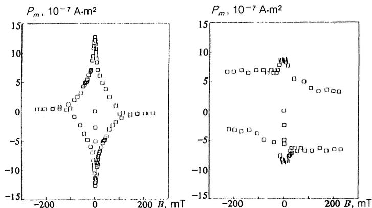
FIG. 5. Field dependences of the magnetic moment of the single crystal  $\kappa$ -(BEDT-TTF)<sub>2</sub>Cu[N(CN)<sub>2</sub>]Cl<sub>0.5</sub>Br<sub>0.5</sub>,  $T = 4.2$  K: a) **B**⊥*bc*, b) **B**||*bc*.
