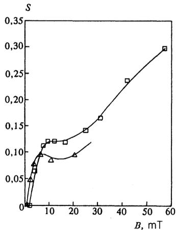
FIG. 9. Field dependences of the relaxation rate  $S = d(\ln P_m^*) / d(\ln t)$ ,  $T = 4.2$  K,  $\mathbf{B} \perp bc$ :  $\square$ — $\kappa$ -(ET)<sub>2</sub>Cu[N(CN)<sub>2</sub>]Cl<sub>0.5</sub>Br<sub>0.5</sub>;  $\triangle$ — $\kappa$ -(ET)<sub>2</sub>Cu(NCS)<sub>2</sub>.
