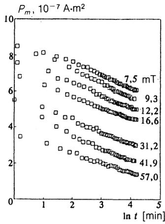
FIG. 8. Time dependences of the magnetic moment of the single crystal  $\kappa$ -(BEDT-TTF)<sub>2</sub>Cu[N(CN)<sub>2</sub>]Cl<sub>0.5</sub>Br<sub>0.5</sub>,  $T = 4.2$  K,  $\mathbf{B} \perp bc$ .
