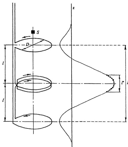
FIG. 1. Second order gradient meter of the flux transformer of the SQUID magnetometer. The solid line shows the calculated dependence of the SQUID-magnetometer response on the displacement of the sample along the  $z$  axis of the gradient meter. The points show experimental values,  $S$  marks the position of the sample.
