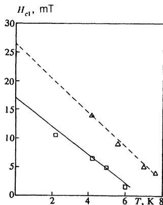
FIG. 4. Temperature dependences of the first critical field of the single crystals  $\kappa$ -(ET)<sub>2</sub>X [X = Cu(NCS)<sub>2</sub> (Δ), Cu[N(CN)<sub>2</sub>]Cl<sub>0.5</sub>Br<sub>0.5</sub> (□)] at an orientation **B**⊥*bc*.
