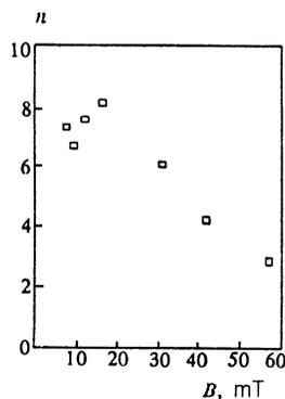
FIG. 12. Dependence of  $n = d(\ln E)/d(\ln j)$  on  $B$  for the single crystal  $\kappa$ -(BEDT-TTF)<sub>2</sub> Cu[N(CN)<sub>2</sub>]Cl<sub>0.5</sub>Br<sub>0.5</sub>.
