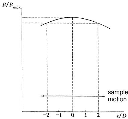
FIG. 2. Field distribution along the gradient meter in the SQUID magnetometer.<sup>6,8</sup>
