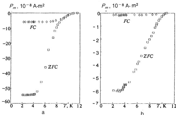
FIG. 3. Temperature dependences of the magnetic moment of the single crystal  $\kappa$ -(BEDT-TTF)<sub>2</sub>Cu[N(CN)<sub>2</sub>]Cl<sub>0.5</sub>Br<sub>0.5</sub>: a)  $\mathbf{B} \perp bc$ ,  $B = 2.1$  mT,  $\square$ —ZFC,  $\diamond$ —FC; b)  $\mathbf{B} \parallel bc$ ,  $B = 1.2$  mT,  $\square$ —ZFC,  $\diamond$ —FC.
