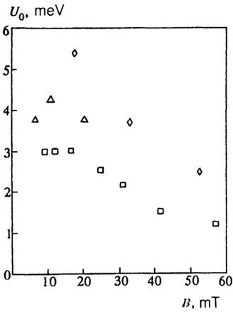
FIG. 10. Field dependences of the average activation energy  $U_0$  at  $T = 4.2$  K:  $\square$ — $\kappa$ -(ET)<sub>2</sub>Cu[N(CN)<sub>2</sub>]Cl<sub>0.5</sub>Br<sub>0.5</sub>,  $\mathbf{B} \perp bc$ ;  $\triangle$ — $\kappa$ -(ET)<sub>2</sub>Cu(NCS)<sub>2</sub>,  $\mathbf{B} \perp bc$ ;  $\diamond$ — $\kappa$ -(ET)<sub>2</sub>Cu(NCS)<sub>2</sub>,  $\mathbf{B} \parallel bc$ .
