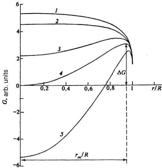
FIG. 1. Thermodynamic potential  $G$  in a particle of radius  $R$  for different values of the magnetic field  $H$ :  $H = 0$  (1),  $H = H^*$  (2),  $H^* < H < H^{**}$  (3),  $H = H^{**}$  (4), and  $H > H^{**}$  (5).
