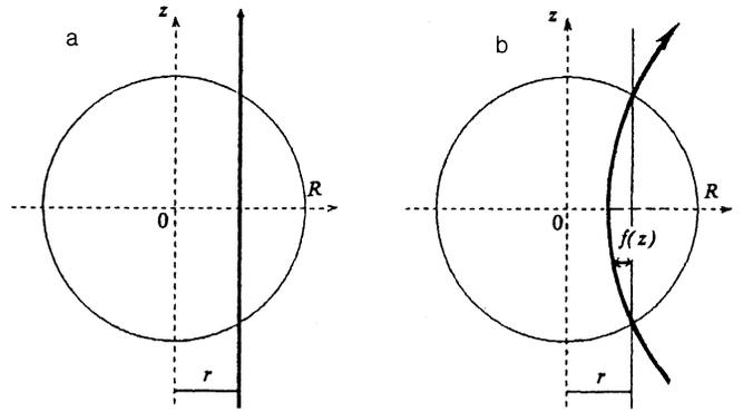
FIG. 2. Vortex filament in a sphere: rectilinear flux line (a) and curved flux line (b).
