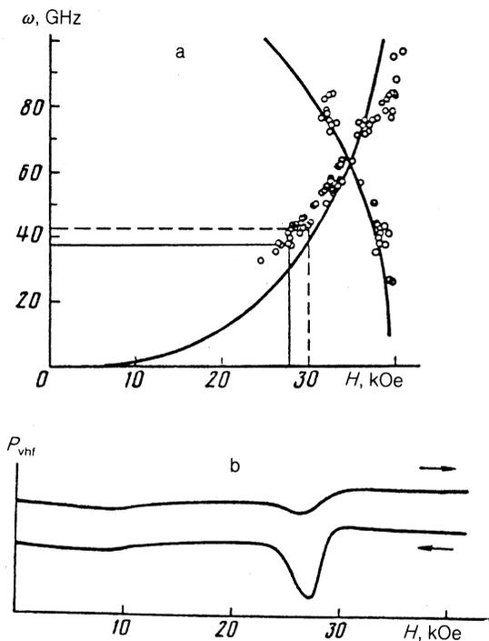
FIG. 3. a—AFMR spectrum in  $\text{RbMnBr}_3$  at  $T = 1.3$  K, field perpendicular to the  $C_6$  axis. The regions of resonance frequencies are shown where "hysteresis" phenomena are observed. b—Example of the trace of the magnetic field dependence of the vhf signal power passing through the resonator containing the specimen for a frequency  $\omega = 36.7$  GHz.
