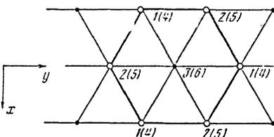
FIG. 1. Distorted crystal structure of  $\text{RbMnBr}_3$  with space symmetry  $C_{6v}^{(1)}$ . The numbers in brackets refer to the positions of Mn ions situated at a distance  $\pm c/2$  from the plane of the drawing.
