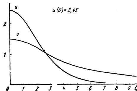
FIG. 1. Field distribution ( $u$ ) and plasma wave potential ( $v$ ) in the self-similar mode.
