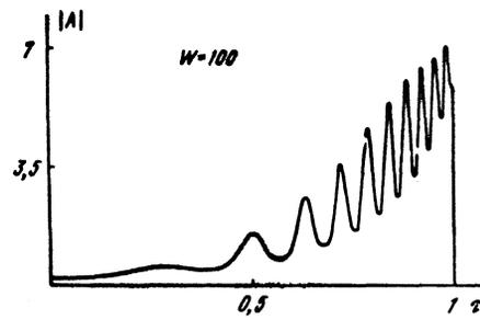
FIG. 2. On-axis field distribution ( $v_{\perp} = 0$ ) for a pulse of rectangular form when  $z = 2$ .
