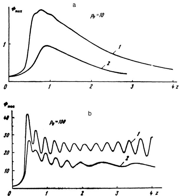
FIG. 4. Dependence of the maximum on-axis plasma wave amplitude ( $v_1 = 0$ ) on the location of the point where it is excited by a pulse of Gaussian shape.
