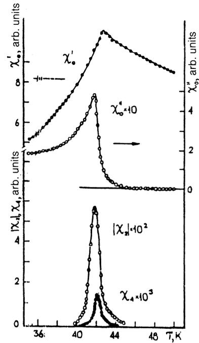
FIG. 1. Temperature dependence of the real component  $\chi'_0$  and the imaginary component  $\chi''_0$  of the dynamic magnetic susceptibility and of the nonlinear susceptibility components  $\chi_2$  and  $\chi_4$  for the alloy ( $\text{Fe}_{0.65}\text{Mn}_{0.35}$ ) $_{75}\text{P}_{16}\text{B}_6\text{Al}_3$ . The amplitude of the magnetization-reversal field is 1 Oe, and its frequency is 83.7 Hz.
