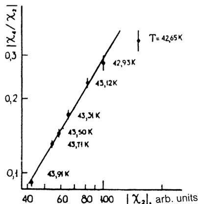
FIG. 2. Plot of  $|\chi_4/\chi_2|$  versus  $|\chi_2|$  for the amorphous alloy ( $\text{Fe}_{0.65}\text{Mn}_{0.35}$ ) $_{75}\text{P}_{16}\text{B}_6\text{Al}_3$ .
