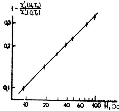
FIG. 5. Field dependence of the parameter  $1 - \chi_0'(H, T_m) / \chi_0'(0, T_f)$  for the spin glass  $(\text{Fe}_{0.65}\text{Mn}_{0.35})_{75}\text{P}_{16}\text{B}_6\text{Al}_3$ .
