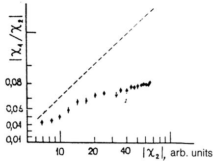
FIG. 7. Plot of  $|\chi_4/\chi_2|$  versus  $|\chi_2|$  for the crystalline alloy  $\text{Fe}_{56}\text{Ni}_{24}\text{Cr}_{20}$ . The dashed line corresponds to  $\beta/\gamma = 0$ .
