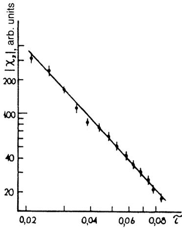
FIG. 3. Nonlinear magnetic susceptibility  $\chi_2$  versus the reduced temperature  $\tau$  for the alloy  $(\text{Fe}_{0.65}\text{Mn}_{0.35})_{75}\text{P}_{16}\text{B}_6\text{Al}_3$ .
