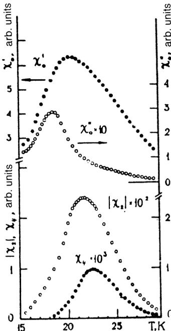
FIG. 6. Temperature dependence of the real component  $\chi'_0$  and the imaginary component  $\chi''_0$  of the dynamic magnetic susceptibility and of the nonlinear susceptibility components  $\chi_2$  and  $\chi_4$  for the crystalline alloy  $\text{Fe}_{56}\text{Ni}_{24}\text{Cr}_{20}$ . The amplitude of the magnetization-reversal field is 1 Oe, and its frequency is 83.7 Hz.
