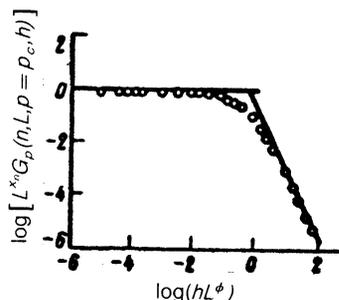
FIG. 3. Multifractal moment of a percolation sample for  $n=3, d=2$ : Monte Carlo results from Ref. 7. The straight lines correspond to the weak-link model.
