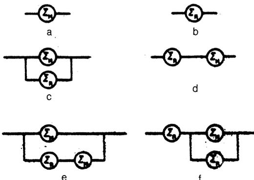
FIG. 2. Equivalent electrical circuits of the steps in the hierarchy.
