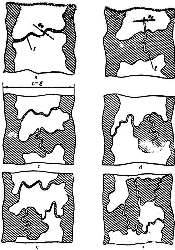
FIG. 1. Hierarchical weak-link model. The phase with good conductivity is hatched. 1—bridge, 2—interlayer,  $a_0$ —minimum size of the structure (in the lattice model—the link length); a, c, e, (b, d, f) are the first, second, and third steps in the hierarchy, which correspond to the first term, first two terms, and first three terms in Eqs. (2) and (3), respectively.
