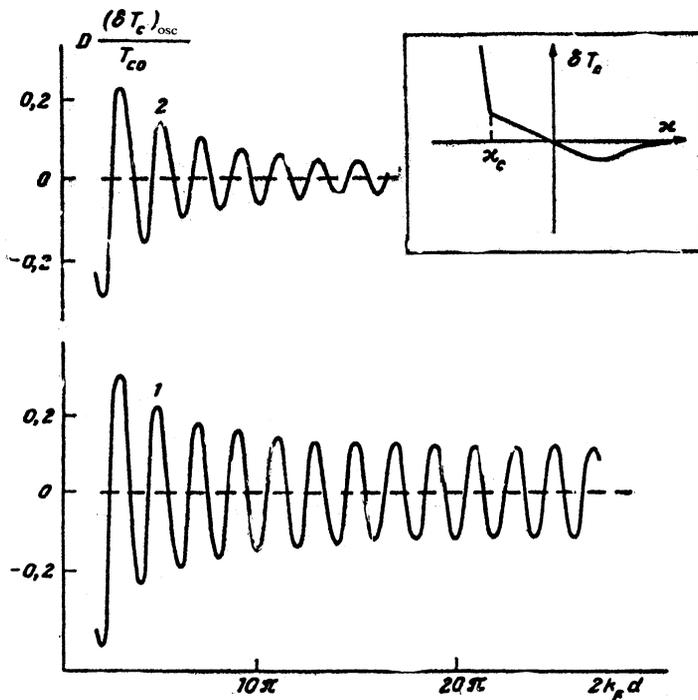
FIG. 4. Form of quantum oscillations near transition  $|\kappa - \kappa_c| \ll \kappa_c$ , curve 1— $\kappa > \kappa_c$ , curve 2— $\kappa < \kappa_c$ . The inset shows  $T_c$  versus  $\kappa$  for a single defect; here  $D = \lambda_0 k_F L / \pi$ .
