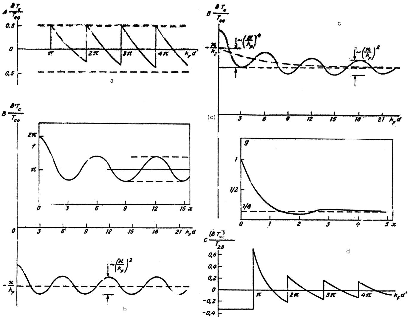
FIG. 2. Form of the quantum oscillations for the geometry in Fig. 1b with different ratios of  $\kappa$  and  $k_F$ : a)  $\kappa \gg k_F$ , b)  $0 < \kappa \ll k_F$ , c)  $\kappa < 0$ ,  $|\kappa| \ll k_F$ , d)  $\kappa < 0$ ,  $|\kappa| \gg k_F$ ; here  $A = \lambda_0 k_F L / \pi$ ,  $B = \lambda_0 k_F L$ , and  $C = (\pi/16)^2 (|\kappa|/k_F)^5 \lambda_0 k_F L$ .
