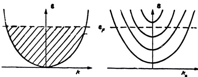
FIG. 3. For  $\kappa \gg k_F$  there are two independent subsystems: the three-dimensional system for  $|z| > d/2$  with a continuous spectrum (on the left) and a quasi-two-dimensional system for  $|z| < d/2$ , whose spectrum consists of a collection of two-dimensional bands (on the right).
