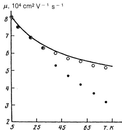
FIG. 4. The temperature curves representing the theoretical results (solid line) and experimental data<sup>10</sup> for the electron mobility in HgSe:Fe samples with  $N_{\text{Fe}} = 5.3 \cdot 10^{19} \text{ cm}^{-3}$ . The experimental values of  $\mu$  are depicted without the phonon contribution (O) and with the phonon contribution (●).
