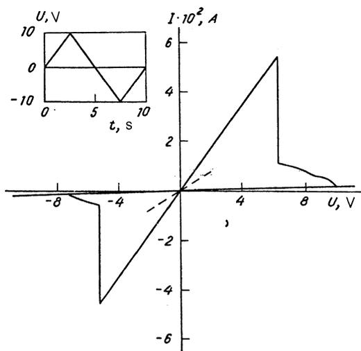
FIG. 3. Current-voltage characteristic of a polymer film under a uniaxial pressure of 0.1 MPa. A bipolar sawtooth voltage with a frequency of 0.1 Hz and an amplitude of  $\pm 10$  V is applied to the sample. The dashed line separates regions corresponding to the half-period of increasing voltage and the half-period of decreasing voltage. The inset shows the voltage waveform applied to the sample.
