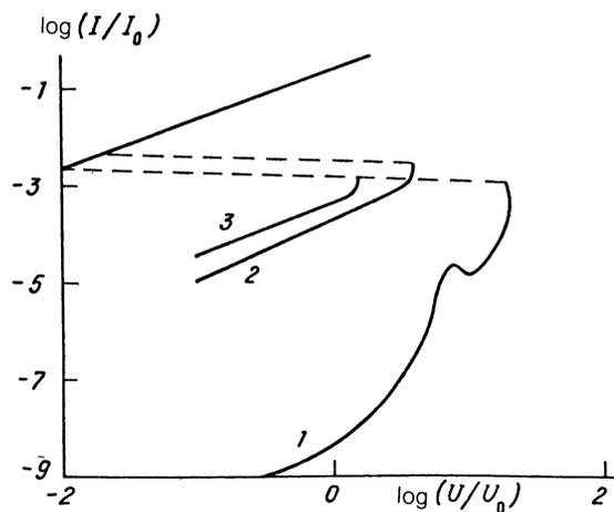
FIG. 2. Current-voltage characteristics of a thin polymer film. 1—In the original insulating state; 2—under a pressure of 0.4 MPa; 3—in the “intermediate” state after a “switching off” by a current pulse.
