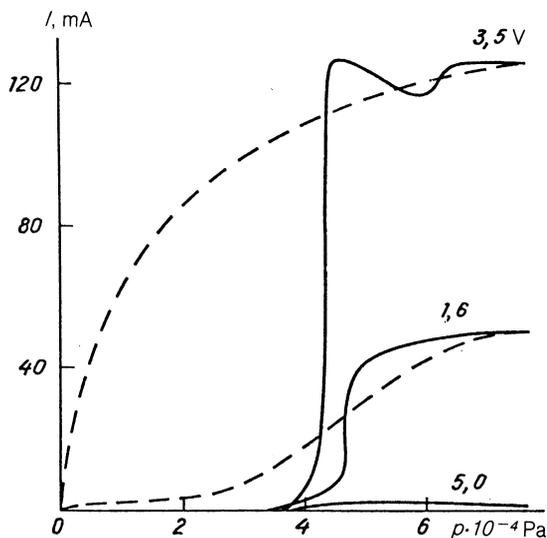
FIG. 1. Current through a polymer film  $0.5 \mu\text{m}$  thick versus the uniaxial pressure.
