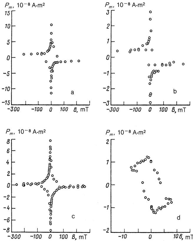
FIG. 2. Magnetization curves of a  $k$ -(BEDT-TTF) $_2$ Cu[N(CN) $_2$ ]Br single crystal for the orientation  $B \perp bc$  ( $bc$  is the conducting plane of the crystal): a)  $T = 2.1$  K, crystal No. 1; b)  $T = 4.2$  K, crystal No. 1; c)  $T = 6.5$  K, crystal No. 1; d)  $T = 4.2$  K, crystal No. 2.
