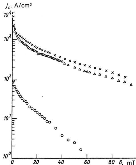
FIG. 5. Field dependence of the critical current density in  $k$ -(BEDT-TTF)<sub>2</sub>Cu[N(CN)<sub>2</sub>]Br single crystals (No. 1) for the orientation  $B \perp bc$ :  $T = 2.1$  K (×), 4.2 K (Δ), and 6.5 K (○).
