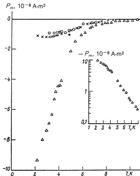
FIG. 1. Temperature dependence of the magnetic moment of  $k\text{-(BEDT-TTF)}_2\text{Cu}[\text{N}(\text{CN})_2]\text{Br}$  single crystals for the orientation  $B \perp bc$ :  $\Delta$ —ZFC,  $B = 3.5$  mT, crystal No. 1;  $\circ$ —FC,  $B = 3.5$  mT, crystal No. 1;  $\times$ —ZFC,  $B = 3.5$  mT, crystal No. 2.
