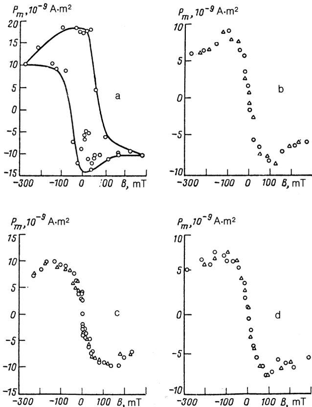
FIG. 3. Magnetization curves of a  $k$ -(BEDT-TTF) $_2$ Cu[N(CN) $_2$ ]Br single crystal for the orientation  $B \parallel bc$  (crystal No. 1):  $T = 2.1$  K (a), 4.2 K (b), 5.7 K (c), and 7.1 K (d).  $\circ$  for b,c,d corresponds to the increase of  $B$ , and  $\triangle$  corresponds to its decrease.
