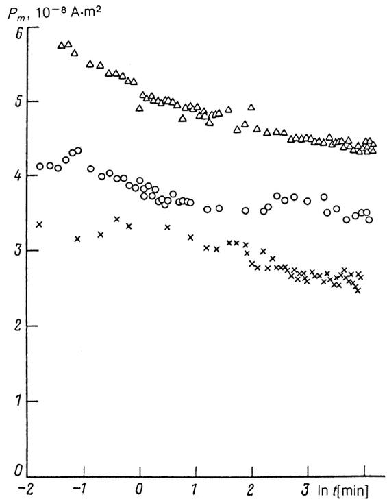
FIG. 7. Time dependence of the magnetic moment  $P_m$  of single crystal No. 2  $k$ -(ET) $_2$ Cu[N(CN) $_2$ ]Br at  $B = 3 \text{ mT}$  ( $\Delta$ ),  $4.6 \text{ mT}$  ( $\circ$ ), and  $7.6 \text{ mT}$  ( $\times$ ).
