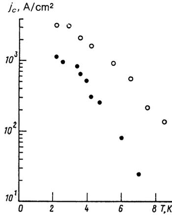
FIG. 4. Temperature dependence of the critical current density in  $k$ -(BEDT-TTF)<sub>2</sub>Cu[N(CN)<sub>2</sub>]Br single crystals for the orientation  $B \perp bc$ ,  $B \rightarrow 0$ ; ●—crystal No. 2, ○—No. 1.
