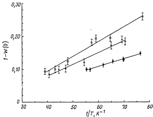
FIG. 2. Temperature dependence of the  $\gamma$  anisotropy of oriented  $^{60}\text{Co}$  nuclei in  $\text{Pd}_{99}\text{Co}_1$ . + — Sample saturated with hydrogen at a pressure of 4 Pa; ■ — the same, but at a pressure of  $2.5 \cdot 10^4$  Pa; □ — sample annealed in vacuum.
