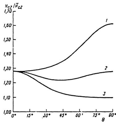
FIG. 3. The angular dependence of the upper critical field  $H_{c2}(\theta)$  in the units of  $H_{c2}^0 = ac\zeta/(2|e|K_4)$  for  $\varepsilon = 0.33$ ,  $\mu = 0$  and  $K_4/K_1 = 0.85$ ; 1.37; and 1.85 (curves 1, 2, and 3, respectively).
