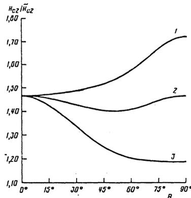
FIG. 4. The angular dependence of the upper critical field  $H_{c2}$  for  $\varepsilon = 0.33$ ,  $\mu = -0.1$  and  $K_4/K_1 = 0.75$ ; 1.05; and 1.58 (curves 1, 2, and 3, respectively).
