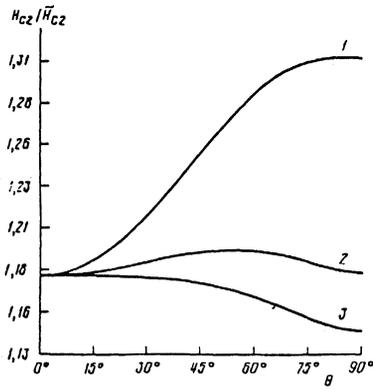
FIG. 5. The angular dependence of  $H_{c2}$  for  $\varepsilon = 0.1$ ,  $\mu = 0.15$  and  $K_4/K_1 = 0.72$ ;  $0.89$ ; and  $0.94$  (curves 1, 2, and 3, respectively).
