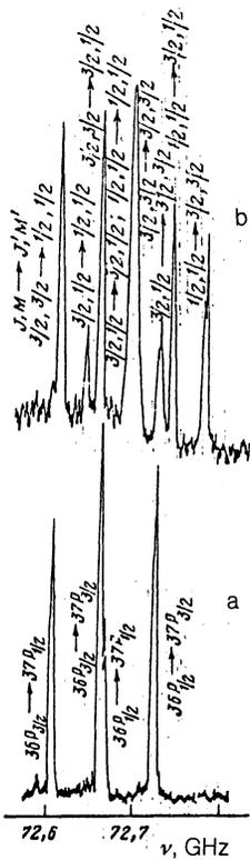
FIG. 7. Experimental observation of the influence of the static Stark effect on the spectrum of the two-photon transition  $36P-37P$  in the Na atom. a— $E = 0$ ; b— $2.2$  V/cm. The microwave intensity is  $I \approx 10^{-7}$  W/cm $^2$ .
