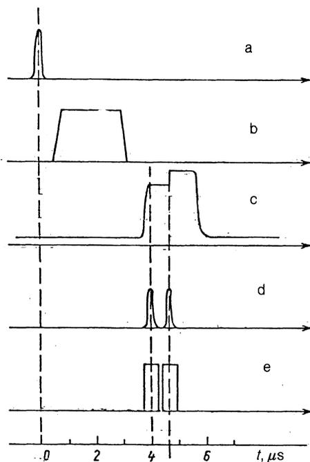
FIG. 3. Time diagram of the excitation and detection pulses. a—Laser pulse; b—microwave field pulse; c—doubled field-ionization pulse; d—electronic pulses representing the densities of atoms in the upper and lower working states; e—strobe pulses in the signal processing.
