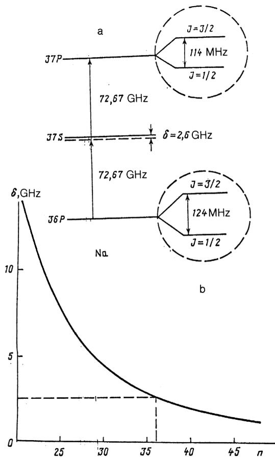
FIG. 1. a—Scheme of two-photon  $nP \rightarrow (n+1)P$  transitions in Na Rydberg atoms with allowance for the fine structure; b—detuning of the real intermediate  $(n+1)S$  level and the virtual level of the two-photon transition along the frequency scale versus the main quantum number  $n$ .
