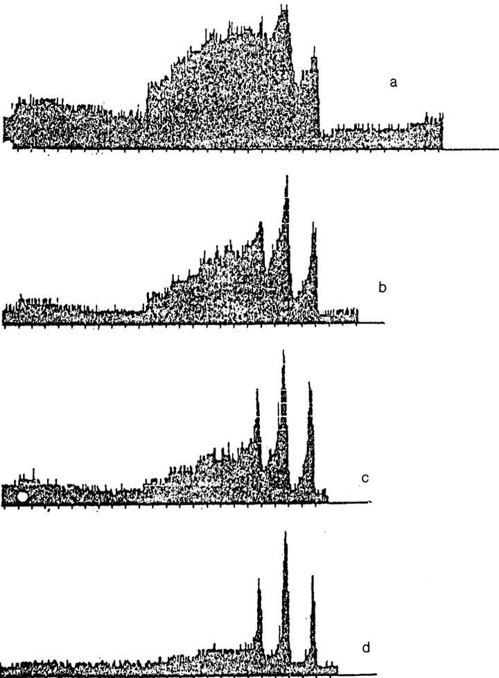
FIG. 5. Field-induced broadening of the spectra of the two-photon absorption on the  $36P \rightarrow 37P$  transition for various microwave intensities. a— $10^{-3}$  W/cm<sup>2</sup>; b— $4 \cdot 10^{-4}$ ; c— $2.5 \cdot 10^{-4}$ ; d— $10^{-4}$  W/cm<sup>2</sup>. These recordings were generated in the course of processing in a CAMAC and DVK-3 complex.
