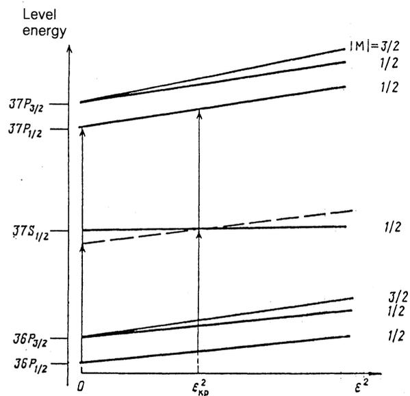
FIG. 6. Splitting of Rydberg levels of Na in a static electric field in the model of the quadratic Stark effect, along with a physical picture of the appearance of a double Stark resonance on the  $nP \rightarrow (n+1)P$  transitions. a— $E=0$ ; b—2.2 V/cm.
