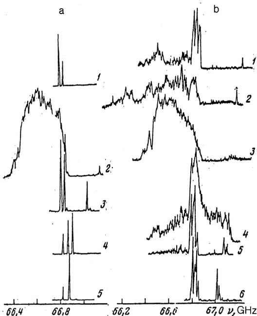
FIG. 11. Appearance of a double Stark resonance on the  $37P \rightarrow 38P$  two-photon transition. a: Total Stark spectrum of the transition.  $I-E = 6.6$  V/cm; 2—5.5; 3—4.4; 4—2.2; 5—0 V/cm. b: Frequency shift of the double resonance at low frequencies.  $I-E = 6.08$  V/cm; 2—5.81; 3—5.53; 4—5.25; 5—5.00; 6—4.42 V/cm.
