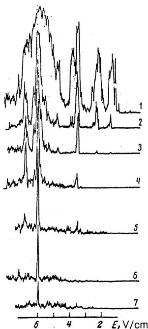
FIG. 10. Experimental spectrum of the double Stark resonance recorded as the electric field was swept at a fixed microwave frequency, 72.9 GHz 1—The microwave intensity is  $8 \cdot 10^{-6}$  W/cm<sup>2</sup>; 2— $4 \cdot 10^{-6}$ ; 3— $2 \cdot 10^{-6}$ ; 4— $8 \cdot 10^{-7}$ ; 5— $4 \cdot 10^{-7}$ ; 6— $8 \cdot 10^{-8}$ ; 7— $4 \cdot 10^{-8}$  W/cm<sup>2</sup>.
