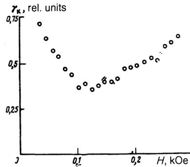
FIG. 5. Dependence of the phonon relaxation rate in  $\text{CoCO}_3$  on the static magnetic field:  $\mathbf{H} \parallel \text{EA}$ ,  $T = 1.97$  K,  $\omega_p/2\pi = 1446$  MHz.
