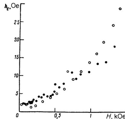
FIG. 6. Dependence of the perpendicular pumping threshold in  $\text{CoCO}_3$  on the static magnetic field at the two directions of  $\mathbf{H}$ :  $\bullet$ — $\mathbf{H} \parallel \text{EA}$ ,  $T = 1.94$  K,  $\omega_p/2\pi = 1430$  MHz;  $\circ$ — $\mathbf{H} \perp \text{EA}$ ,  $T = 1.5$  K,  $\omega_p/2\pi = 1570$  MHz.
