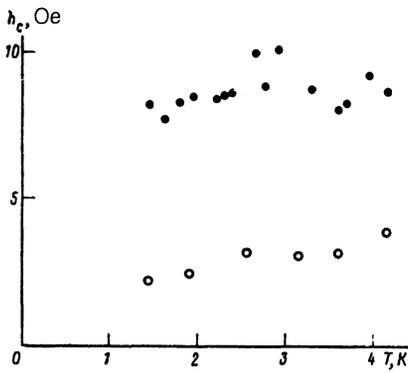
FIG. 7. Temperature dependences of the phonon parametric excitation thresholds in  $\text{CoCO}_3$ : ●— $\mathbf{H} \parallel \mathbf{h} \parallel \mathbf{EA}$ ,  $\omega_p/2\pi = 1570$  MHz,  $H = 155$  Oe; ○— $\mathbf{H} \perp \mathbf{h} \parallel \mathbf{EA}$ ,  $\omega_p/2\pi = 1570$  MHz,  $H = 274$  Oe.
