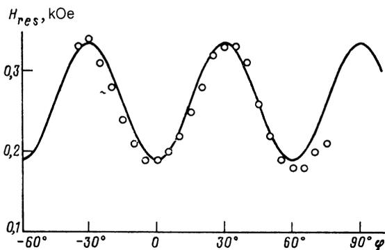
FIG. 1. Dependence of the resonant AFMR magnetic field on direction in the basal plane of the  $\text{CoCO}_3$  crystal. The angles  $\varphi = 0^\circ$  and  $\varphi = 60^\circ$  correspond to  $\mathbf{H} \parallel \text{EA}$ ;  $T = 4.2$  K,  $\omega_{f_0}/2\pi = 16.63$  GHz. The solid curve was calculated according to the formula  $H [\text{Oe}] = 262 - 73 \cos 6\varphi$ .
