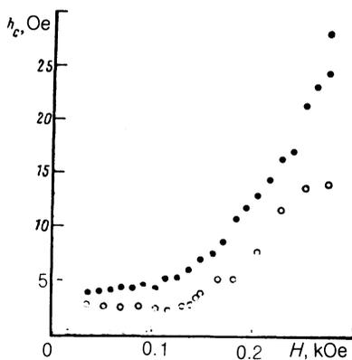
FIG. 4. Dependence of the parallel pumping threshold in  $\text{CoCO}_3$  on the static magnetic field at the two directions of  $\mathbf{H}$ :  $\bullet$ — $\mathbf{H} \parallel \text{EA}$ ,  $T = 1.97$  K,  $\omega_p/2\pi = 1446$  MHz;  $\circ$ — $\mathbf{H} \perp \text{EA}$ ,  $T = 1.94$  K,  $\omega_p/2\pi = 1430$  MHz.
