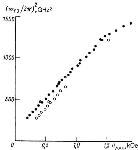
FIG. 2. Square of the AFMR frequency in  $\text{CoCO}_3$ , as a function of the static magnetic field  $H$  for two directions of the field in the basal plane:  $\bullet$ — $\mathbf{H} \parallel \text{EA}$ ,  $\circ$ — $\mathbf{H} \perp \text{EA}$ ,  $\Delta$ —data of Ref. 19;  $T = 4.2$  K.
