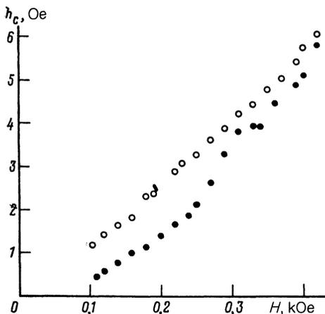
FIG. 8. Dependence of the phonon parametric excitation threshold in  $\text{FeBO}_3$  on the static magnetic field for the two pumping geometries: ●— $\mathbf{H} \parallel \mathbf{EA} \parallel \mathbf{h}$ , ○— $\mathbf{H} \perp \mathbf{EA} \parallel \mathbf{h}$ ;  $T = 77$  K,  $\omega_p/2\pi = 620$  MHz.
