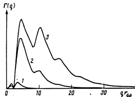
FIG. 1. The phonon absorption coefficient versus the phonon wave vector for the parameter  $r_\omega/a$  equal to 2(1), 6(2) and 10(3).
