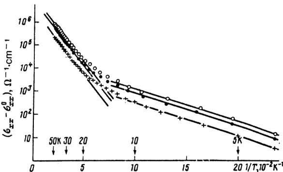
FIG. 4. Temperature dependence of the electron magnetoconductivity of sample No. 1 for  $H = 60$  (○), 75 (●), and 140 kOe (+) for  $\mathbf{H} \parallel \langle 110 \rangle$ .
