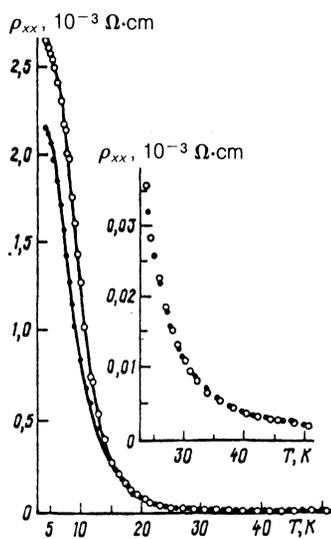
FIG. 2. Dependence of the magnetoresistance  $\rho_{xx}(T)$  on temperature when  $H = 140$  kOe. (O)— $\mathbf{H} \parallel \langle 111 \rangle$ ; (●)— $\mathbf{H} \parallel \langle 110 \rangle$ . In the inset we show high-temperature segments of these curves, in expanded scale.
