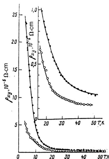
FIG. 7. Temperature dependence of the Hall resistivity of sample Nos. 3 and 4 (●)— $\mathbf{H}\langle 111 \rangle$ ; (○)— $\mathbf{H}\langle 110 \rangle$  for  $H = 140$  kOe. The inset shows in an expanded scale the high-temperature segments of these curves.
