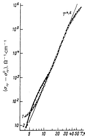
FIG. 3. Temperature dependence of the electron magnetoconductivity of tungsten samples Nos. 1 and 2 ( $\sigma_{xx}(T) - \sigma_{xx}^0$ ) in base 10 logarithmic coordinates when  $H = 140$  kOe: (O)— $\mathbf{H} \parallel \langle 111 \rangle$ ; (●)— $\mathbf{H} \parallel \langle 110 \rangle$ .
