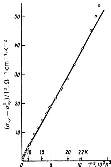
FIG. 6. Temperature dependence of the electron magnetoconductivity of sample No. 2 for  $T < 20 \text{ K}$ ,  $H = 140 \text{ kOe}$ ,  $\mathbf{H} \parallel \langle 111 \rangle$ .
