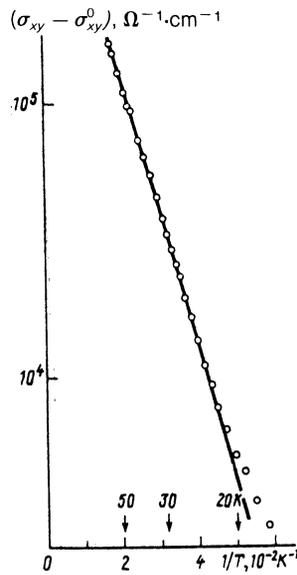
FIG. 5. Temperature dependence of the electron magnetoconductivity of sample No. 2 for  $T > 20 \text{ K}$ ,  $H = 140 \text{ kOe}$ ,  $\mathbf{H} \parallel \langle 111 \rangle$ .
