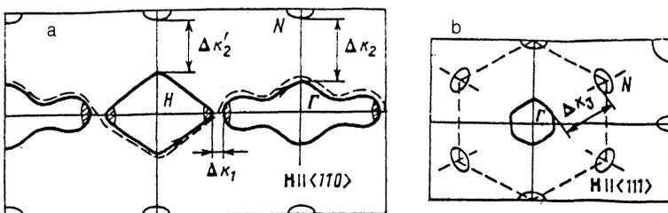
FIG. 1. Extremal cross sections of the Fermi surface of tungsten: (a) the plane (110); (b) the plane (111).  $\Delta k_1$ ,  $\Delta k_2$ ,  $\Delta k'_2$ , and  $\Delta k_3$  are the gaps between sheets of the Fermi surface.
