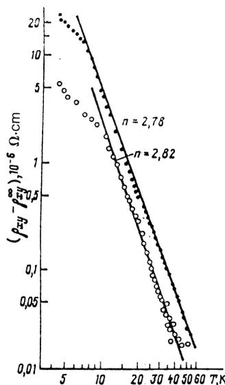
FIG. 8. Temperature dependence of the Hall resistivity of sample Nos. 3 and 4 for  $H = 140$  kOe (●)— $\mathbf{H} \parallel \langle 111 \rangle$ ; (○)— $\mathbf{H} \parallel \langle 110 \rangle$ . For the meaning of  $\rho_{xy}^{\infty}$  consult the text.
