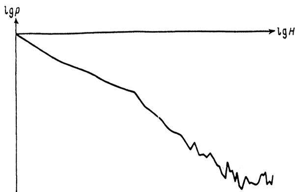
FIG. 3. Probability density versus the magnetic field, in logarithmic scale. The approximately linear shape of this distribution supports the contention that the distribution is not Gaussian. The parameter values are the same as for Fig. 2a.
