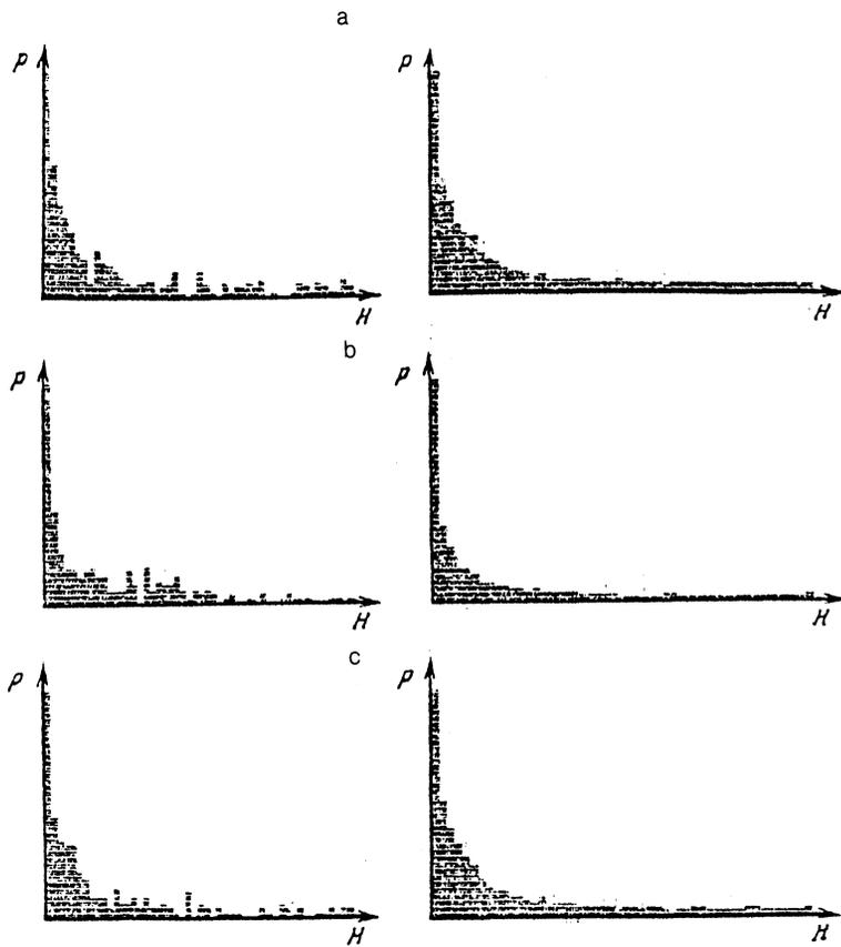
FIG. 2. Probability density of the magnetic field distribution. Left: Snapshot at the time  $n = 39$ . Right: Average over 20 time steps (from the 22nd to the 41st). The magnetic diffusion coefficient  $\varepsilon$  is (a) 0.5 or (b) 3. The nonlinearity in (3) is quadratic in the magnetic field. c—Probability density for a cubic nonlinearity with a diffusion coefficient 0.5.
