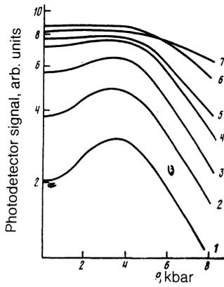
FIG. 2. The pressure dependence of the emission intensity for pressure  $P \parallel [100]$  in intermediate electric fields ( $E$ , V/cm): 6 (1), 10 (2), 15 (3), 20 (4), 40 (5), 60 (6), and 100 (7).
