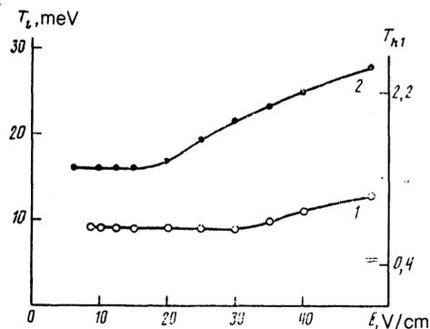
FIG. 5. Temperatures of light holes ( $T_l$ ) and heavy holes ( $T_h$ ) for different crystallographic directions:  $[111]$  (1) and  $[100]$  (2).
