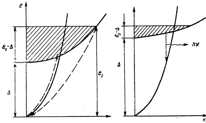
FIG. 8. Diagram illustrating the onset of strong inversion with band splitting by an amount of the order of the energy of an optical phonon.
