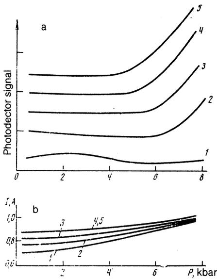
FIG. 7. Pressure dependence ( $P \parallel [111]$ ) of the intensity of spontaneous emission (a) and of the current flowing through the specimen (b) for different electric fields  $E$  (in kV/cm): 0.6 (1), 1.0 (2), 2.0 (3), 3.0 (4), and 4.0 (5).
