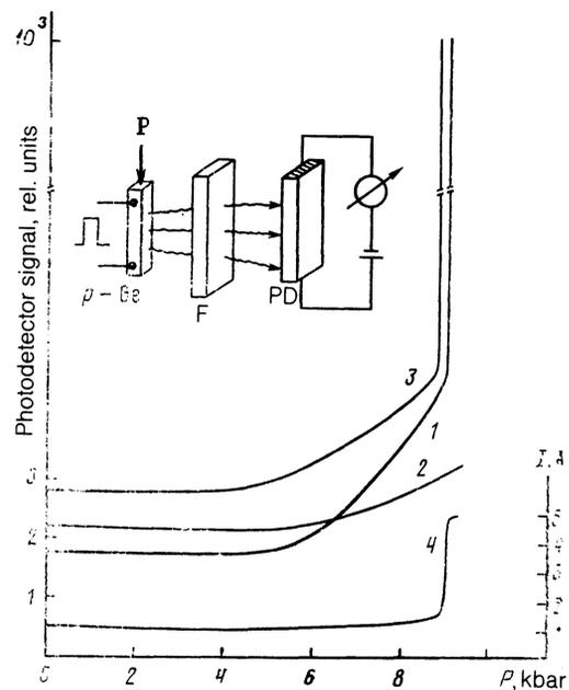
FIG. 1. Arrangement of the experiment (a) and dependence of the emission (1–3) and current (4) on the pressure  $\mathbf{P} \parallel [111]$ : 1, 4) initial specimen; 2) after rough grinding; 3) after repeated polishing; F—filter; PD—photodetector.
