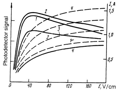
FIG. 3. The photodetector signal (solid lines) and the current flowing through the specimen (dashed lines) as a function of the electric field for different pressures  $P \parallel [111]$ : 0 (1), 1.8 (2), 3.6 (3), and 5.0 (4) kbar.
