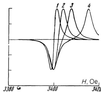
FIG. 6. Calculated derivative of the absorption curves for various magnetic field gradients  $k$ . 1— $k = 0$ ; 2— $k = 4$  Oe; 3— $k = 8$  Oe; 4— $k = 16$  Oe. In the absence of a gradient ( $k = 0$ ), the resonance field is  $H_0 = 3400$  Oe, and the line width is  $\Delta H = 2$  Oe.
