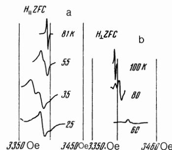
FIG. 4. Representative recordings of the ESR lines during cooling in the residual field of the magnet,  $\approx 20$  Oe (ZFC), for the cases in which the magnetic field is (a) parallel to and (b) perpendicular to the plane of the platelet.
