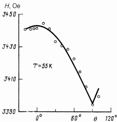
FIG. 1. Orientation dependence of the position of the ESR line found during cooling in the residual field of the magnet,  $\approx 20$  Oe, to  $T = 55$  K (ZFC).
