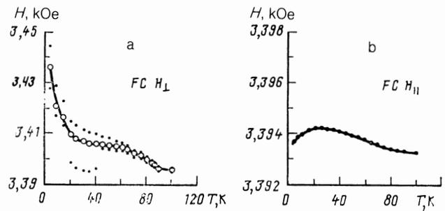
FIG. 3. Temperature dependence of the position of the ESR line found during cooling in the field corresponding to the beginning of the recording,  $\approx 3390$  Oe (FC). a—The field is directed perpendicular to the plane of the platelet; b—parallel to this plane.
