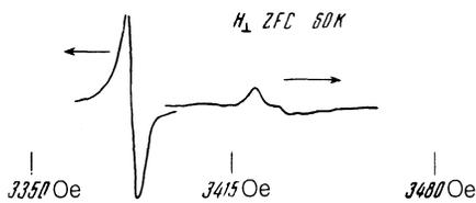
FIG. 5. Demonstration of the sensitivity of the ESR line to the magnetic history of the sample. The high-field line was recorded after the sample was cooled in the residual field of the magnet,  $\approx 20$  Oe, and the field was raised during the recording of the line, to 3500 Oe. The low-field line was recorded during the subsequent decrease of the magnetic field.
