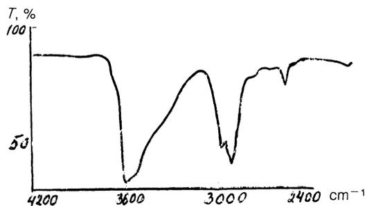
FIG. 3. IR spectrum of the prepared samples of cellulose nitrate. The thickness of the film is equal to  $\approx 30 \mu\text{m}$ .
