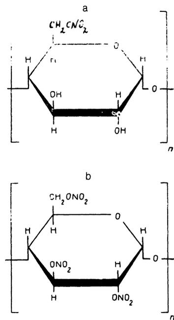
FIG. 2. Structural formulas for monomers of cellulose mononitrate (a) and trinitrate (b).
