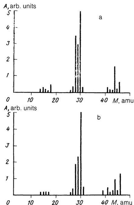
FIG. 4. Mass spectra of the products of dissociation of macromolecules irradiated in the stretching-vibration band of OH groups ( $\lambda = 2.80 \mu\text{m}$ ) (a) and the CH groups ( $\lambda = 3.43 \mu\text{m}$ ) (b).
