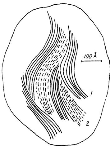
FIG. 1. Schematic diagram of the supermolecular structure of the polymer studied. The different lines show different types of associates of the macromolecules: 1— $[R(ONO_2)_3]_n$  and 2— $[R(OH)_2(ONO_2)]_n$ . Here R is the part of the monomer remaining after substitution and  $n$  is the degree of polymerization.
