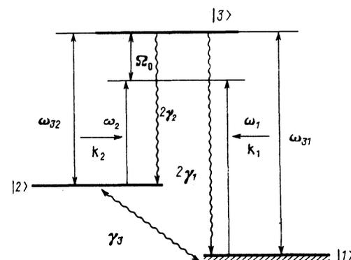
FIG. 1. Interaction of a  $\Lambda$  atom with the field of oppositely directed waves as in (1).
