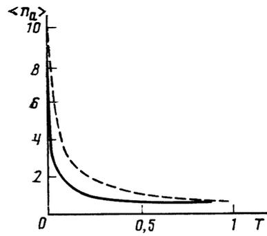
FIG. 2. Time evolution of the average number  $\langle n_a \rangle$ , of photons in the pump mode for an initial value  $\bar{n}_a = 10$ . The dashed line shows the same function in the case of two-photon absorption, again for  $\bar{n}_a = 10$  (Ref. 13).
