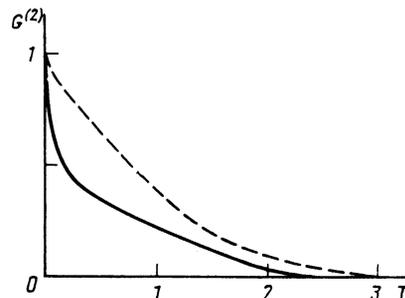
FIG. 3. Time evolution of the factor  $G^{(2)}$  for the pump mode in the cases of (solid line) hyper-Raman scattering and (dashed line) two-photon absorption.<sup>13</sup>
