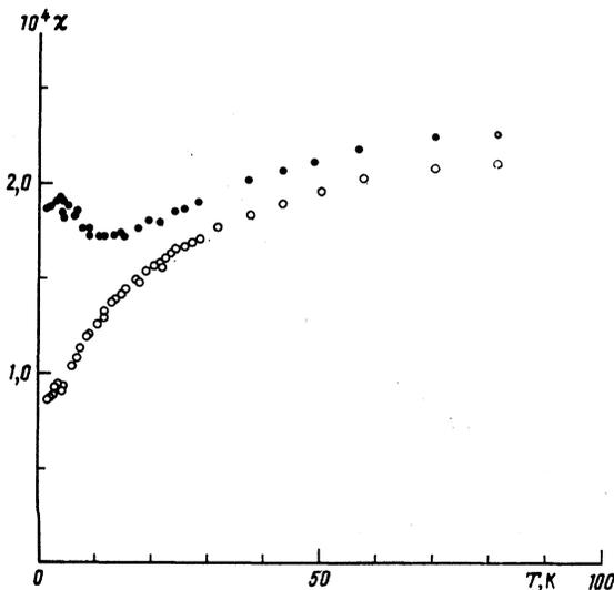
FIG. 3. Temperature dependence of the magnetic susceptibility  $\chi$  of a single crystal for the orientations (●)  $\mathbf{H} \parallel \mathbf{c}$  and (○)  $\mathbf{H} \perp \mathbf{c}$  ( $H = 22.5$  kOe).
