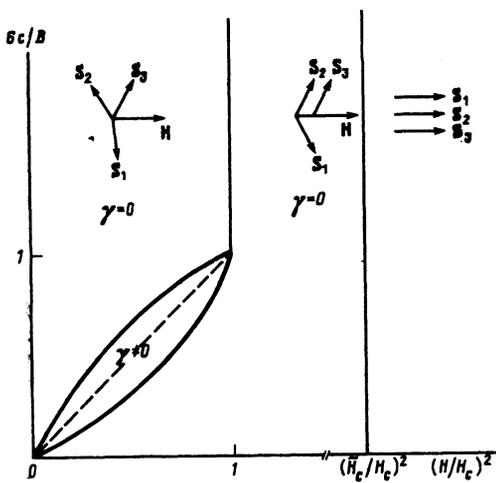
FIG. 8. Phase diagram of crystals of the CsMnBr<sub>3</sub> type in a field H||c as calculated from the thermodynamic potential (8).
