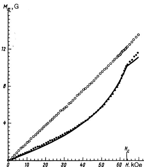
FIG. 2. Field dependence of the magnetizations (O)  $M_{x\parallel}$  and (●)  $M_{x\perp}$  at  $T = 1.7 \text{ K}$ . The solid line is a curve of  $M(H)$  calculated from the theory of Ref. 7.
