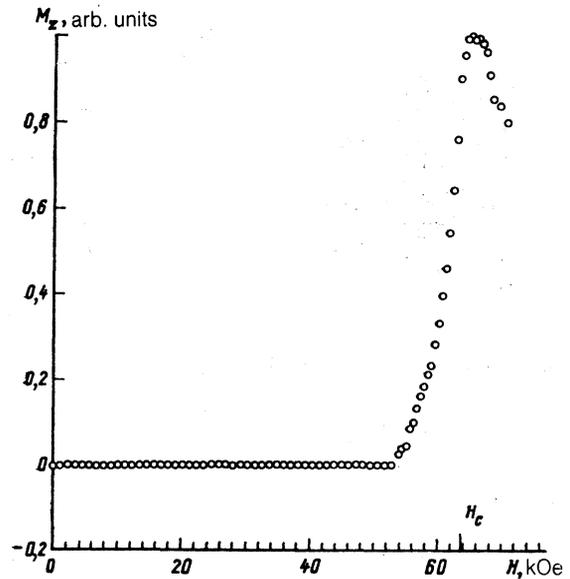
FIG. 4. Field dependence of the magnetization  $M_z \parallel \mathbf{c}$  ( $\mathbf{H} \perp \mathbf{c}$ ,  $T = 1.7$  K).
