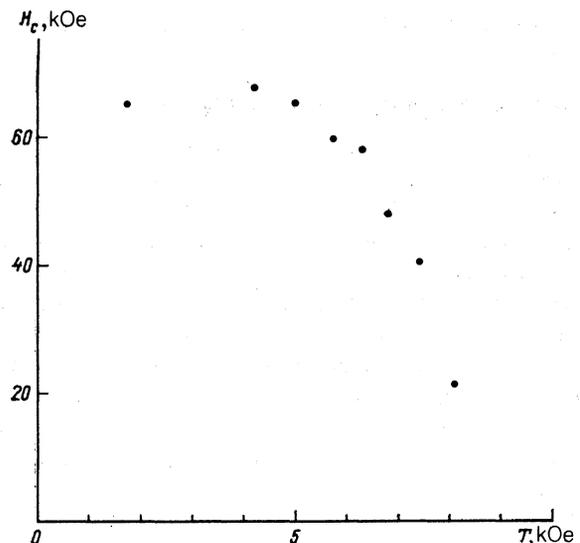
FIG. 5. Temperature dependence of the critical magnetic field  $H_c$  found from the  $M_z(H)$  dependence.
