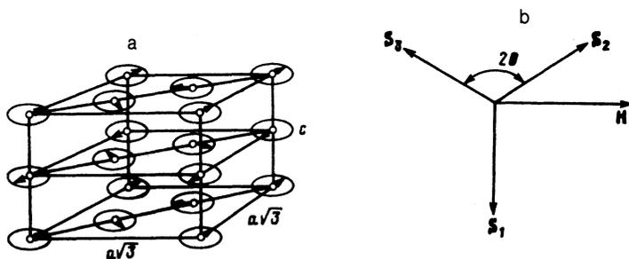
FIG. 1. a—Arrangement of the magnetic moments of the  $Mn^{2+}$  ions in the unit cell of the  $CsMnBr_3$  crystal; b—magnetic moments of the sublattices in one of the basal planes of the crystal as  $H \rightarrow 0$ , brought to a common point.
