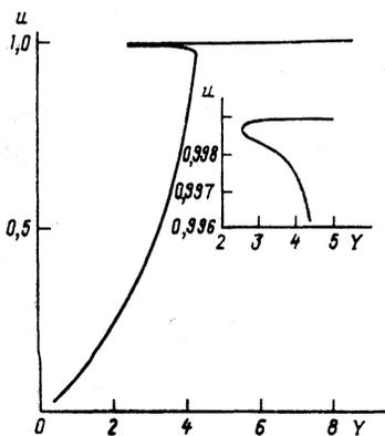
FIG. 2. Density of coherent polaritons  $u$  as a function of pump intensity  $Y$  for a detuning from resonance of  $\Delta\omega/\gamma_{ef} = -3$ .
