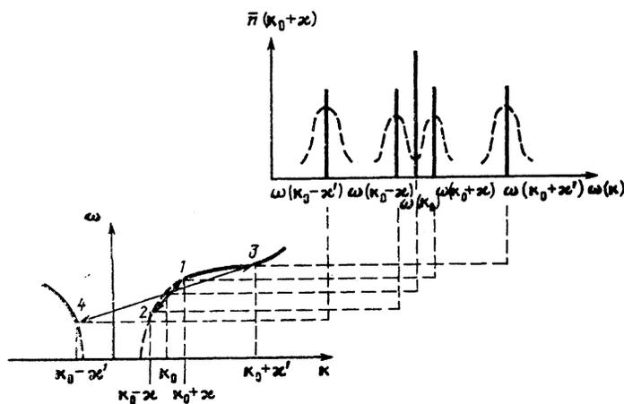
FIG. 1. Dispersion law for the lower polariton band in crystallites and distribution function of scattered polaritons.
