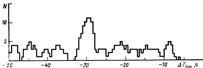
FIG. 1. The distribution of the number of coincidences  $N$  between the events at LSD and at the Baksan telescope, found within one hour, 01:45–02:45 UTC on 23 February 1987, as a function of the shift of the absolute time  $\Delta T_{\text{Bak}}$  (s); the time window of the coincidences is  $\pm 1$  s.
