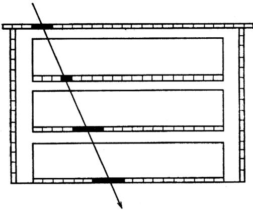
FIG. 6. One of the coincident Baksan events: a muon generating a shower in the telescope. The black blocks denote the detectors which have fired.
