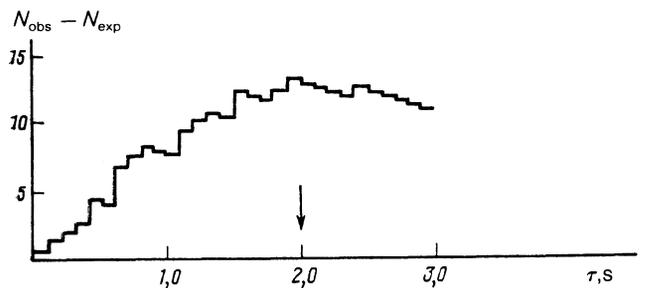
FIG. 5. The excess of observed coincidences  $N_{\text{obs}}$  over expected coincidences  $N_{\text{exp}}$ , between low-energy events at LSD and at the Baksan telescope as a function of the width of the time window  $\tau$ .
