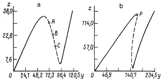
FIG. 2. Various types of "light-light" hysteresis with  $F = 2\pi n$  and (a)  $\delta = 20$  and (b)  $d = 50$  ( $C = 20$ ,  $\varepsilon_\infty = 3.117$ ,  $l/L = 2.94$ ,  $\gamma_{ph}/\gamma_{ex} = 5$ ). The dashed part of the curve corresponds to  $dz/dx < 0$ .
