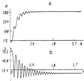
FIG. 5. Dynamics of the switching from the lower branch of the optical-bistability curve to the upper branch for the same parameter values. a—Photons; b—excitons.
