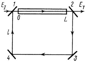
FIG. 1. Ring cavity. Mirrors 1 and 2 have a reflectance  $R$ ; mirrors 3 and 4 have a reflectance of 100%; the distance between mirrors 1 and 2 is  $L$ ; that between mirrors 2 and 3 is  $l$ .
