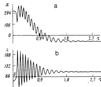
FIG. 4. Dynamics of the switching from the upper branch of the optical-bistability curve to the lower branch for  $C = 40$  and  $\delta = 90$ . a—Photons; b—excitons.
