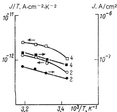
FIG. 6. Temperature dependence of the current in a cell of the  $1 \equiv 1$  type obtained at different voltages. The numbers alongside the curves the voltages in volts.
