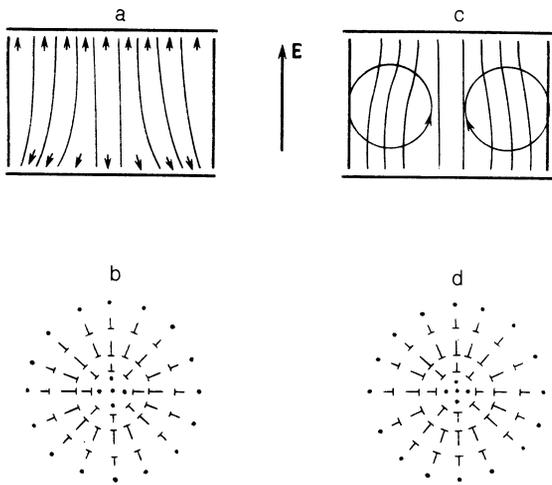
FIG. 1. Geometry of circular domains of the static (a, b) and dynamic (c, d) types in a homeotropically oriented layer of a nematic liquid crystal, induced by the surface polarization and the isotropic electrohydrodynamic mechanisms, respectively. Sections of domains by vertical (a, c) and horizontal (b, d) planes are shown. The arrows identify the directions of the surface polarization (a) and of the vortex flow in the liquid crystal (c).
