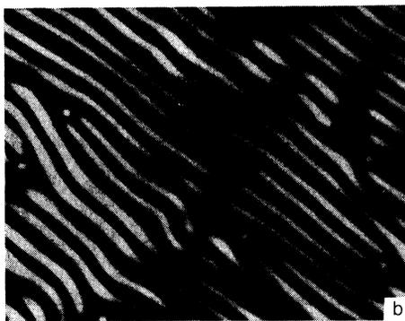
FIG. 3. Photomicrographs of textures of a homeotropically oriented layer of 5CB in cells of the 1 ≡ 1 and 12 ≡ 21 types subjected to a static electric field: a) unrubbed electrode surface; b) rubbed electrode surface.
