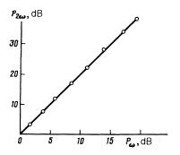
FIG. 2.  $P_{2\omega}(P_{\omega})$  dependence in single crystal YBaCuO at  $T \approx T_c$ ; H||H<sub> $\omega$ </sub>, H = 15 Oe and  $\omega/2\pi = 9.4$  GHz.
