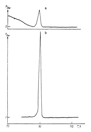
FIG. 1. Dependences of the second-harmonic power  $P_{2\omega}$  on the temperature for ceramic (a) and single-crystal (b) samples of YBaCuO. Frequency  $\omega/2\pi = 9.4$  GHz, external magnetic field H = 20 Oe, the maximum amplitude of the alternating magnetic field  $\mathbf{H}_{\omega} \parallel \mathbf{H}$  on the sample surface is  $H_{z} = 18$  Oe (a) and 15 Oe (b).
