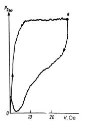
FIG. 3.  $P_{2\omega}(H)$  dependence in single-crystal YBaCuO for  $T \approx T_c$ ;  $H_{\sim} = 10$  Oe and  $\omega/2\pi = 9.4$  GHz. The direction of the current variation was reversed at the point A.
