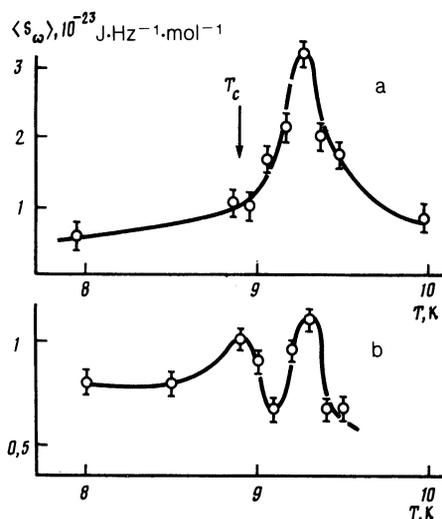
FIG. 4. a) Mean-square power of fluctuations of  $M_{\parallel}$  parallel to the (100) plane component of the magnetic moment in a sample of  $(\text{CH}_3\text{NH}_3)_2 \cdot \text{CuCl}_4$ , averaged over the frequency interval 0.01–10 Hz. b) Same power but for  $M_{\perp}$  when the (100) plane in crystals was perpendicular to the axis of the receiving coil of the superconducting magnetic flux transformer.
