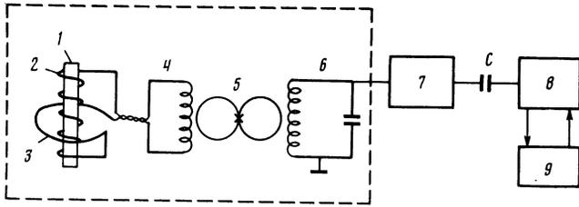
FIG. 1. Block diagram of the flux meter: 1) sample; 2) receiving coil of the flux transformer; 3) compensating coil in the superconducting magnetic flux transformer; 4) signal coil; 5) SQUID sensitive element; 6) hf circuit of the SQUID; 7) electronic unit of the SQUID; 8) digital voltmeter with an input resistance of  $10^8 \Omega$ ; 9) DVK-3 computer. The components enclosed by the dashed box were located directly in the cryostat and kept at liquid helium temperature.
