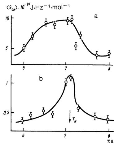
FIG. 7. Temperature dependence of the mean-square power of magnetic fluctuations in  $\text{Mn}_{0.28}\text{Zn}_{0.72}\text{F}_2$  averaged over the frequency intervals 0.01–0.1 Hz (a) and 1–10 Hz (b).
