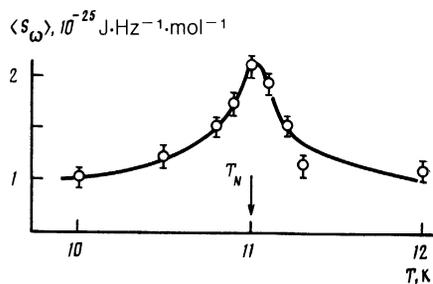
FIG. 3. Temperature dependence of the mean-square power of magnetic fluctuations in  $\text{MnSO}_4$ , averaged over the frequency interval 0.01–10 Hz.
