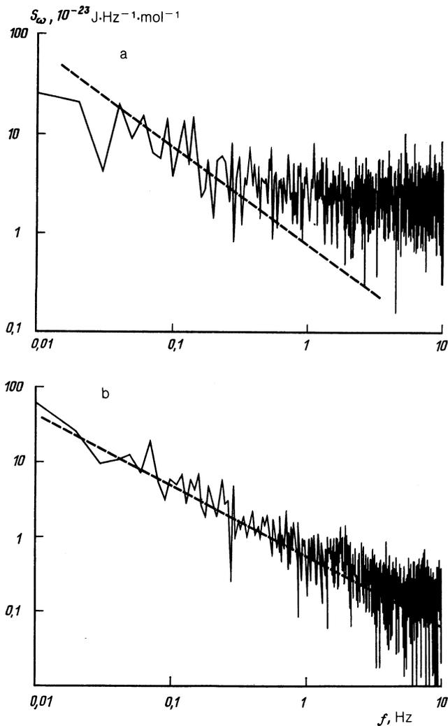
FIG. 8. Spectrum of the magnetic noise in an antiferromagnet of the  $\text{Mn}_{0.28}\text{Zn}_{0.72}\text{F}_2$  composition at temperatures 7.1 K (a) and 6.5 K (b).
