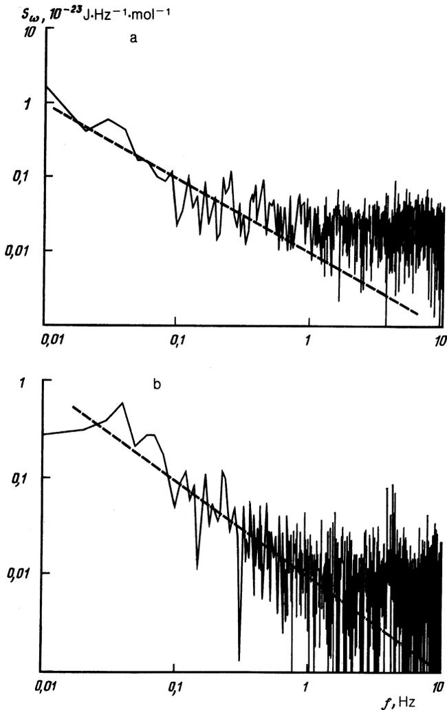
FIG. 5. Frequency dependence of the mean-square power of fluctuations of  $M_{\parallel}$  in  $(\text{CH}_3\text{NH}_3)_2\text{CuCl}_4$  at 9.3 K (a) and in  $\text{K}_2\text{CuF}_4$  at 6.3 K (b). The dashed line represents the  $1/f$  dependence.
