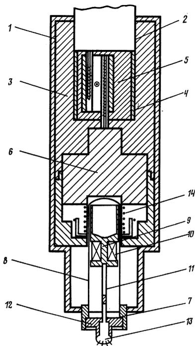
FIG. 2. Construction of the low-temperature unit: 1) copper can; 2) thin-walled tube 16 mm in diameter made of stainless steel; 3), 4) superconducting lead screen; 5) SQUID holder; 6) Teflon holder in the superconducting magnetic flux transformer; 7) platinum tube; 8) test tube; 9) heat conductor; 10) heater; 11) support; 12) flange; 13) bead; 14) receiving coil of the superconducting magnetic flux transformer.
