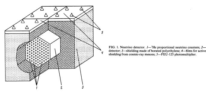
detector; 3-shielding made of borated polyethylene; 4-films for active shielding from cosmic-ray mesons; 5-FEU-125 photomultiplier.
