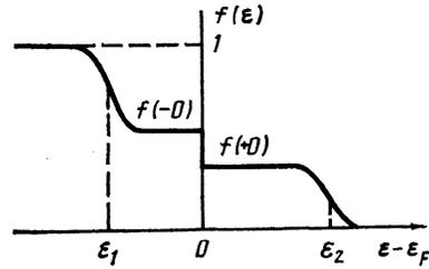
FIG. 2. Electron energy distribution function in a granule at  $T=0$  and high voltages.
