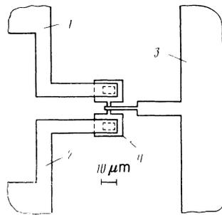
FIG. 1. Schematic diagram of a sample: 1) drain; 2) source; 3) gate; 4) heavily doped regions.
